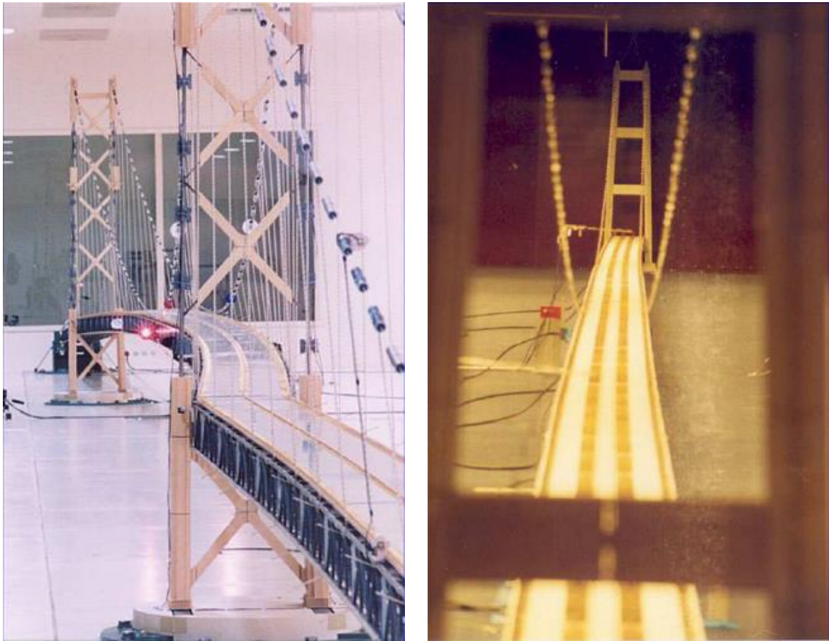
Figure 1.26: Comparison of Akashi-Kaikyo (left) and Messina (right) horizontal deflection due to wind in the wind tunnel.
