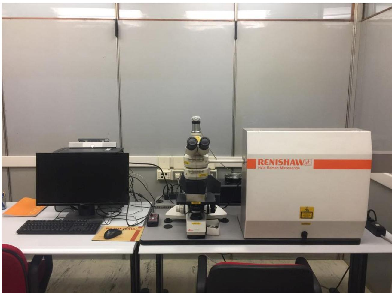
Fig. 3.9 Micro Raman instrument (used for green laser).
