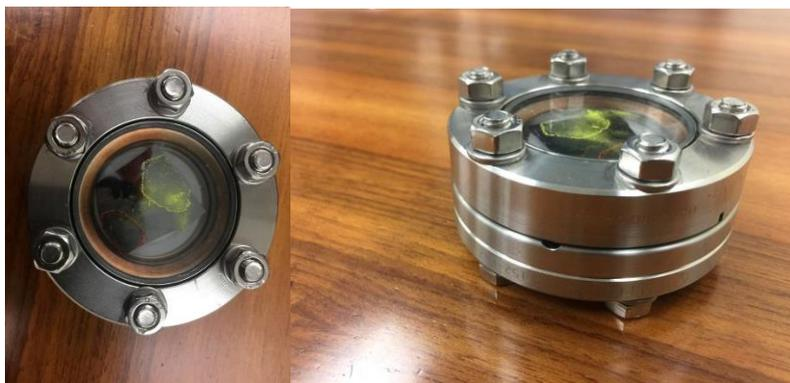
*Fig. 4.5 Ph3 and Ph5 deposited on a silicon substrate locked inside a sealed chamber to perform Raman without exposing to air*
