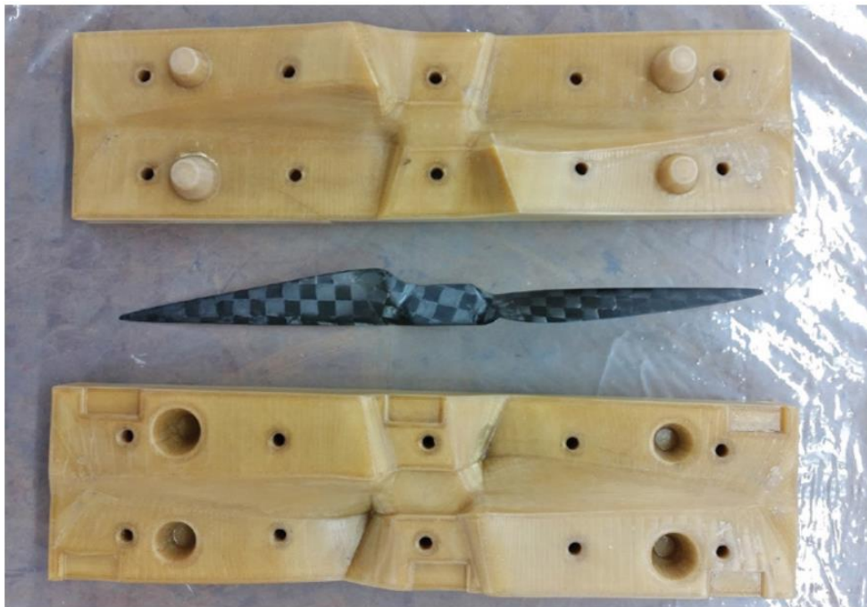
Figure 1.8 Carbon/epoxy UAV propeller manufactured via compression moulding on an Ultem 1010 tool (356x102x102 mm upper and lower molds combined) produced by Stratasys. The total production time was 30 h and the cost was 50% of the estimate for traditional technologies. [50]
