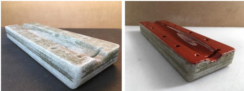
Figure 4.2 The mold after polishing (left) and gelcoat application (right).
