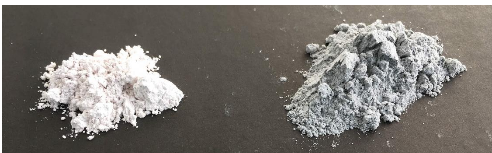
Figure 2.6 Riviera'sca (left) and Gamesa (right) recycled materials. The red hue of Riviera'sca's material and the darker colour of the one supplied by Gamesa are clearly visible.
