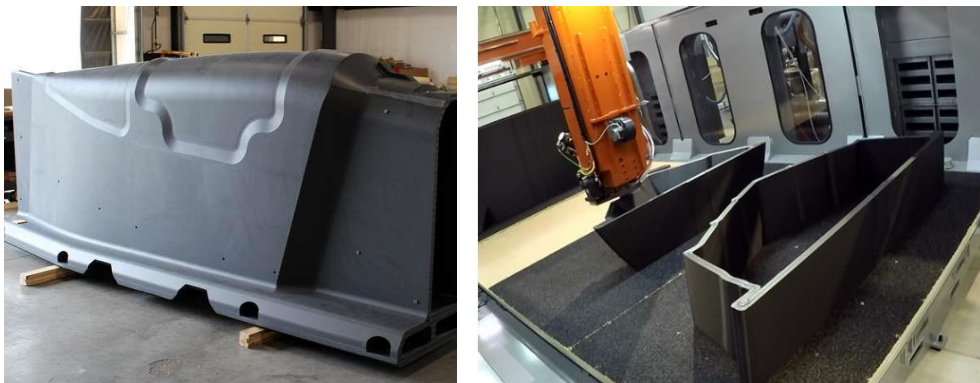
Figure 1.9 Two examples of the LSAM applied to composite tooling. A tool made in collaboration with Boeing for the 777X program and a boat hull mold being fabricated. Both parts are made from ABS with 20 wt% carbon fiber. [46]-[47]
