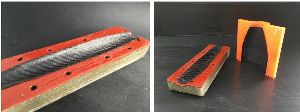
Figure 4.5 The finished mold and part. On the right, comparison with a PETG mold for room temperature applications.
