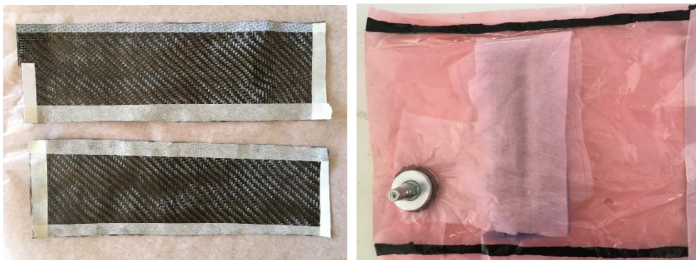
Figure 4.3 Two Hexforce 200 g/m 2 3k 2/2 twill plies and the prepared vacuum bag.
