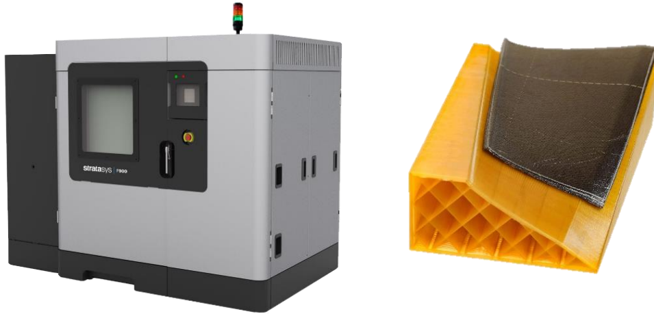
Figure 1.7 Stratasys' Fortus 900 MC FDM 3D printer and an Ultem 1010 tool for the lamination of a winglet printed with it. This hot chamber machine is able to print Stratasys' complete material range and has a 916x610x916 mm build plate. [79]-[80]
