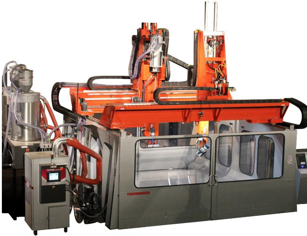
Figure 1.3 Thermwood's LSAM machine. Its build volume is 3 m wide and 1.5 m high and features a modular length that can reach up to 30 m. In addition to the classical extruder, it features a second head equipped with a 5-axis CNC router for machining. [83]
