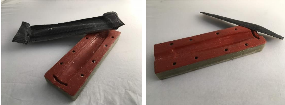
Figure 4.4 Laminated part before (left) and after excess material removal (right).
