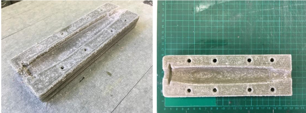
Figure 4.1 The mold immediately after printing (left), with clearly visible residual material deposits, and after their removal (right).
