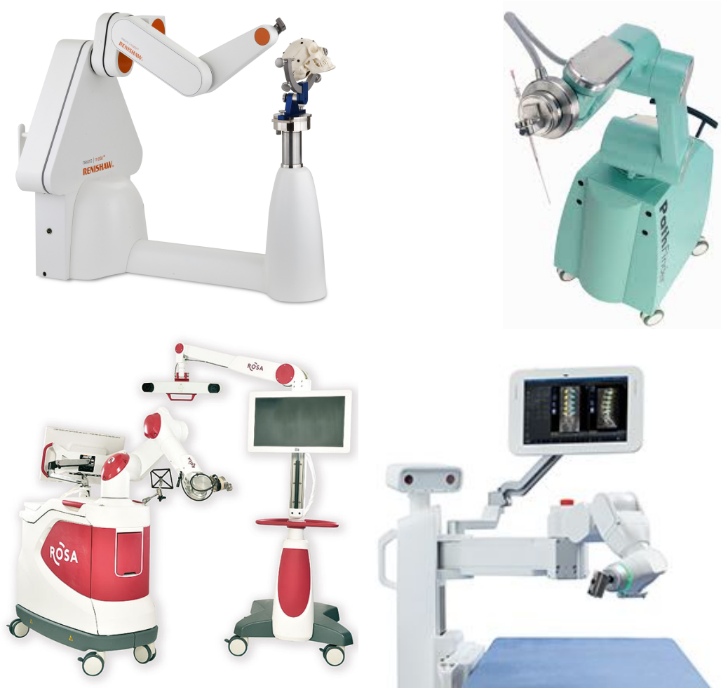
Figure 1.3: Starting from the top left in anticlockwise direction: the Reinshaw Neuromate, the Pathfinder, the ROSA spine, Mazor X.
