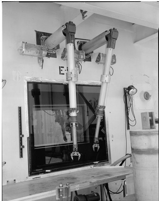
Figure 1.5: Remote manipulator arms designed for the manipulation of radioactive material (Engine Maintenance Assembly & Disassembly Facility, Area 25 of the Nevada Test Site).
