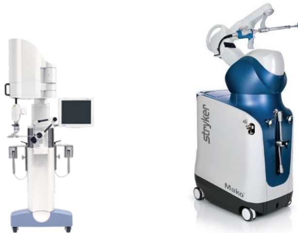
Figure 1.4: From left to right: the TSolution One® system by THINK Surgical and the MAKO system by Stryker for total hip replacement.
