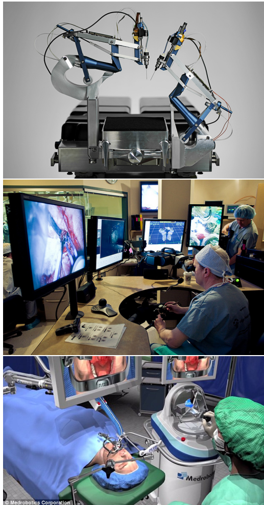
Figure 1.6: From top to bottom: The Preceys system for teleoperated eye surgery, the Neuroarm for teleoperated MRI-compatible neurosurgery and the FLEX endoscopic system.
