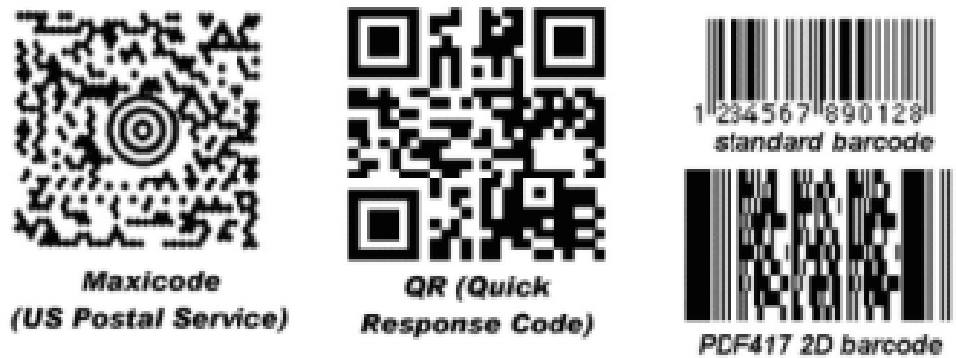
Figure 2.10: Examples of 1D and 2D not fiducial marker systems
