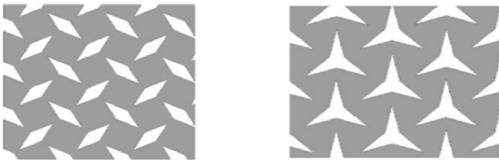
Figure 2.2 Shows the arrangement of shapes leading to Negative Poisson’s ratio
