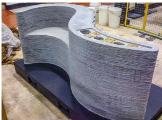
Figure 17 – A full scale bench fabricated by the Concrete Printing with functional voids and posttensioned reinforcement [31]
