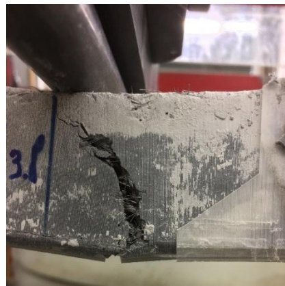
Figure 60 - Cracking in the middle
