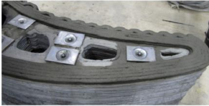
Figure 7 – Digital manufacturing of a free-shaped wall-like concrete bench using the ‘Concrete Printing’ approach
