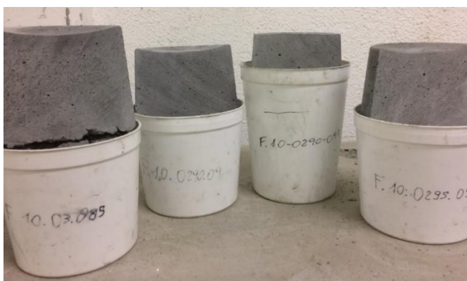
Figure 44 - Best results of High-Performance Fiber Reinforced Concrete cylinder samples
