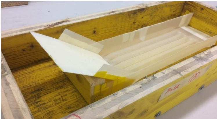
Figure 54 - Ramp in PLA for the Fiber Reinforced Concrete casting
