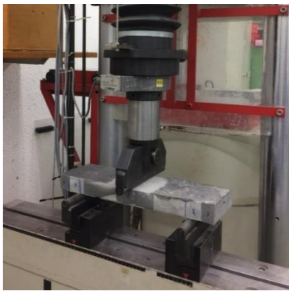
Figure 59 - Setup of the three-point bending test
