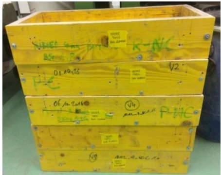
Figure 52 - Wooden formworks, dim. 210 x 60 x 540 mm
