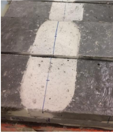
Figure 58 – Surface grinding of the specimens
