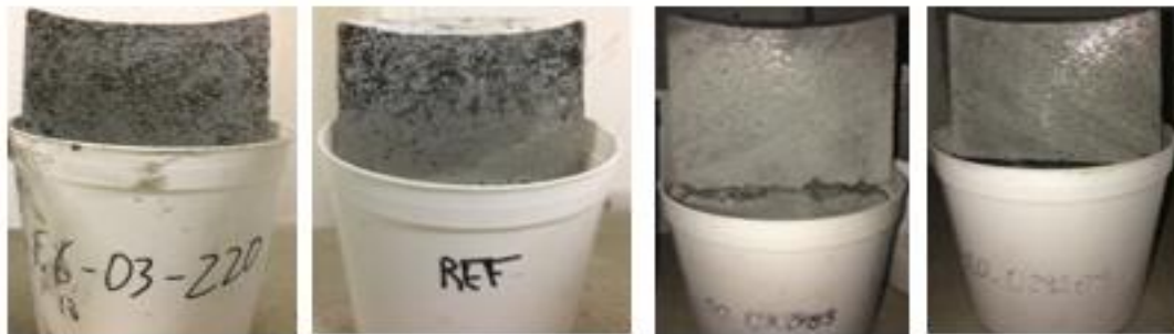
Figure 43 - Segregation of half cylinder samples
