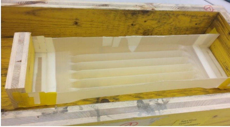
Figure 53 - view of the formwork with double extensions and the piece of wood
