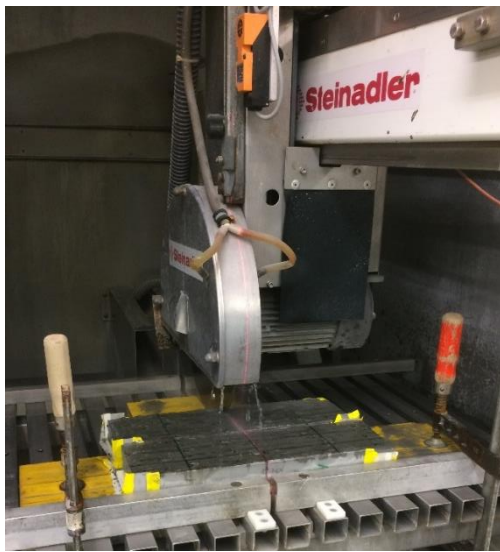
Figure 69 – Cutting machinery and concrete samples in smaller pieces
