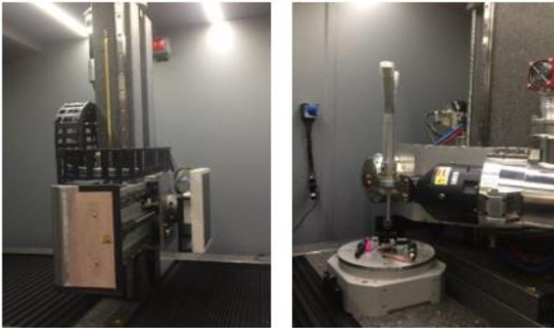
Figure 66 - X-ray computed tomography at EMPA
