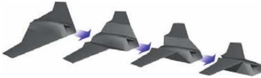
Figura 1.4: Lockheed-Martin Agile Hunter, morphing alare
