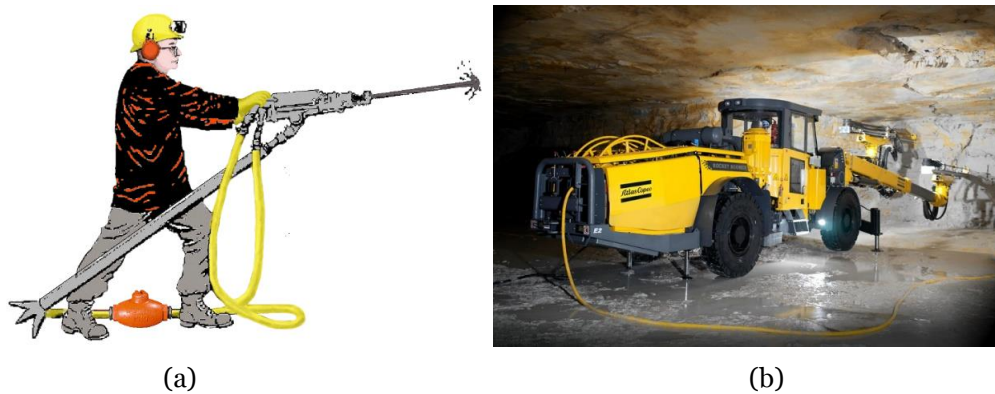
Figure 2 - HAV vibration reduction solution: (a) old methodology: Jack-leg drilling (b) New Technology: Jumbo Drill machine
