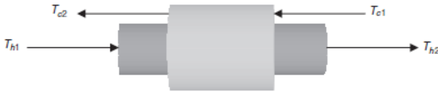
Figure 11. Double-pipe heat exchanger with counter-current flow arrangement with hot fluid flowing in the inner pipe. (Serth, 2007)
