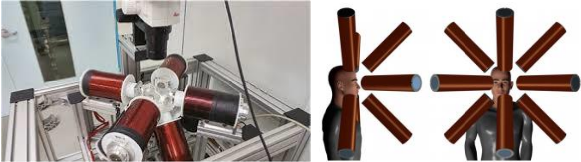
Figure 5.12 - On the left the OctoMag apparatus in ETH Zurich, on the right OctoMag application conceptual layout.
