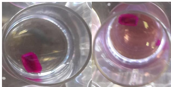
Figure 6.16 - Comparison between Ester bond Rhodamine B Hydrogel before the release (left) and after 1 week (right) at pH 3
