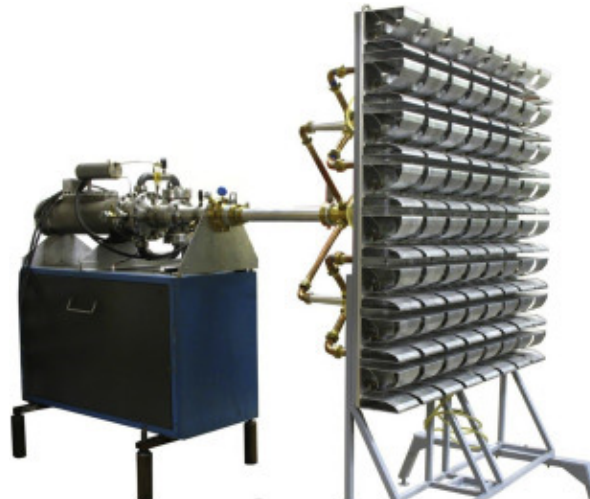
Figure 5. Photo of the UWB electromagnetic radiator with combined antenna array [40] .
