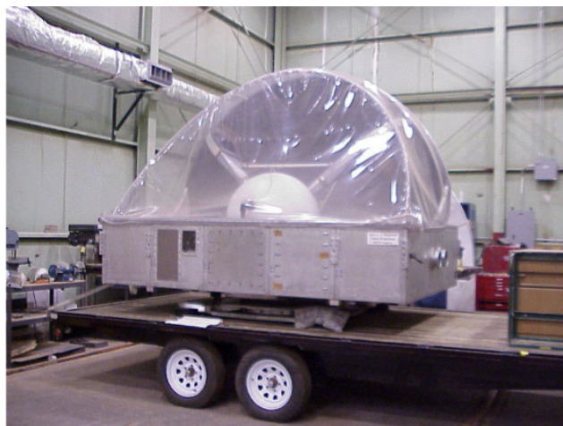
Figure 4. Photo of the “JOLT” UWB electromagnetic radiator [33] .
