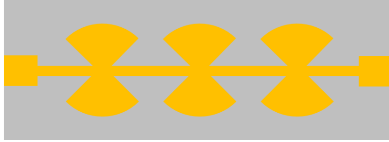
Figure 24. PCB structure of low-pass filter with open-circuited butterfly stubs.
