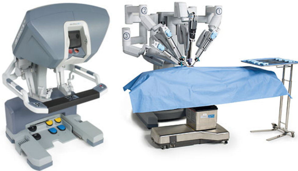
Figure 2.2: Da Vinci : master-slave robotic system for neurosurgeries. The master is on the left side of the image, while the slave is represented on the other side.
