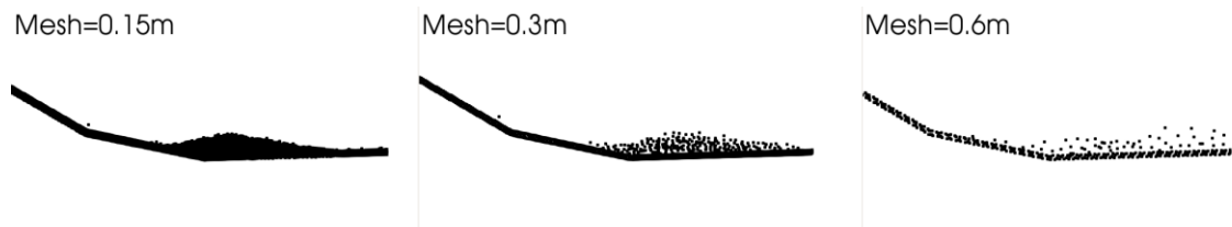
Figure 3.25 Screenshot of the final shape of the deposit for different mesh sizes
