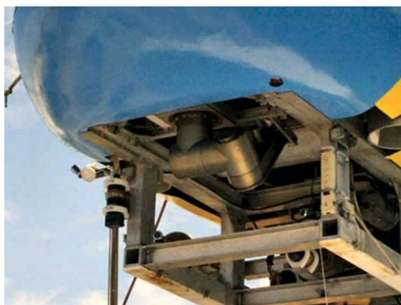
Figure 8 The Enlarged View of Front-end Camera in SAUVIM
