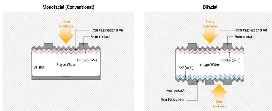
Fig 2.22 Comparison between a conventional cell and a bifacial cell [46].
