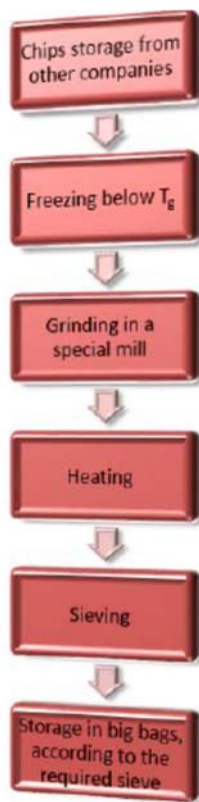
Figure 9.2 – Production scheme of rubber production by Lehigh
