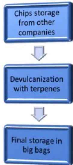
Figure 9.1 – Scheme of production of the rubber powder produced by Austin Rubber
