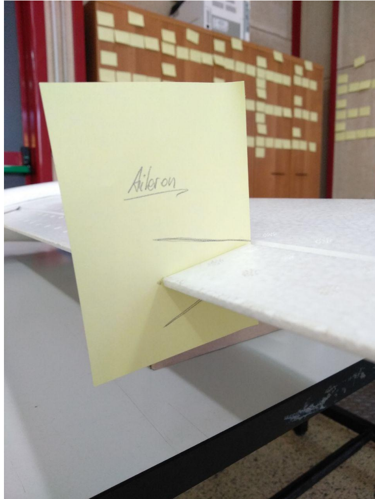
Figure 2.2: Aileron maximum deflection test
