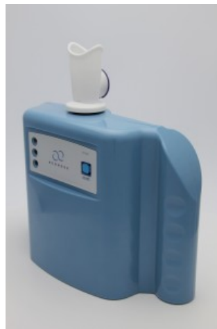
Figure 2.11: The Aeonose device. Image taken from www.enose.nl
