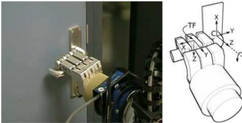
Figure 2.6: Example of physical representation of opening a door through the handle with associated preshape, image taken from [25]
