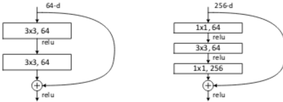
Figure 3.6: ResNet modules, with (right) and without (left) dimensionality reduction inspired by Inception modules, image taken from [51]
