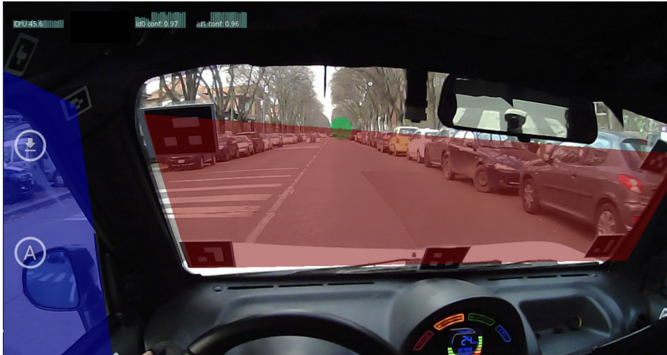
Figure 4.1: An example of detected surfaces: the right window is rarely visible unless the driver is turning right.
