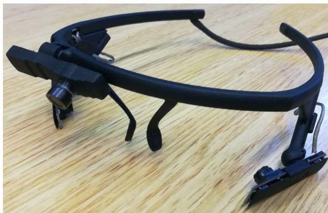
Figure 3.7: Pupil Labs ® eye tracker with two cameras for the eyes and a front camera
