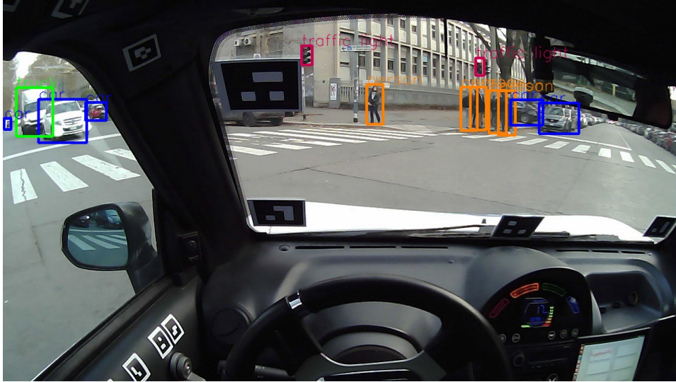
Figure 4.6: A picture of the result of YOLOv3 elaboration during the first acquisition
