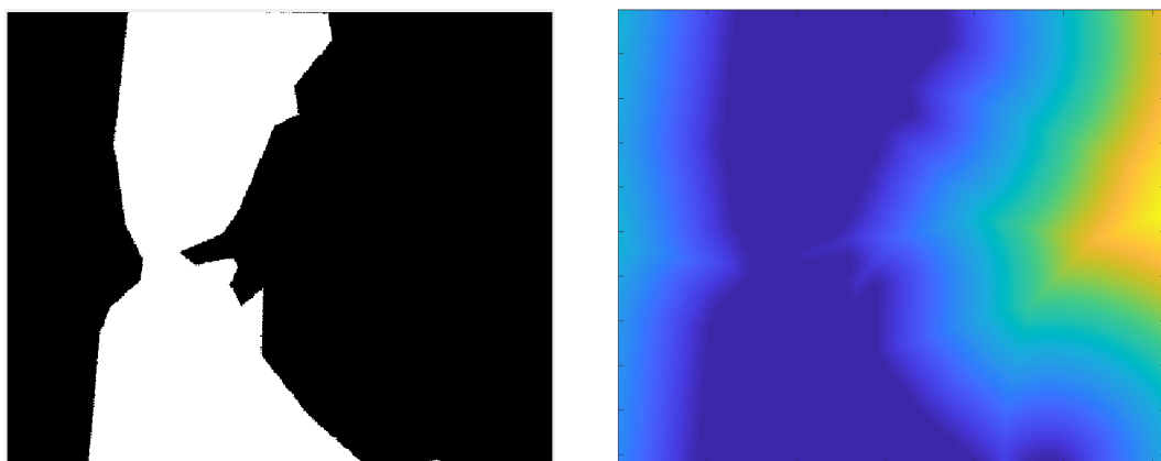
Figure 3.5: Results of the algorithm applied to an image. On the left is presented the river mask, where all the white pixels belong to river, while the black ones do not. On the right is presented the result of the algorithm, where the distance of each pixel from the closest pixel of river is computed. Distance values closer to 0 are in blue, meanwhile higher distance values are in yellow.
