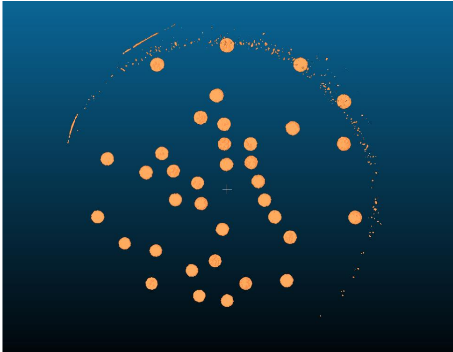
Figure 6.5: Example of the pores after they have been isolated using Matlab and viewed by CloudCompare
