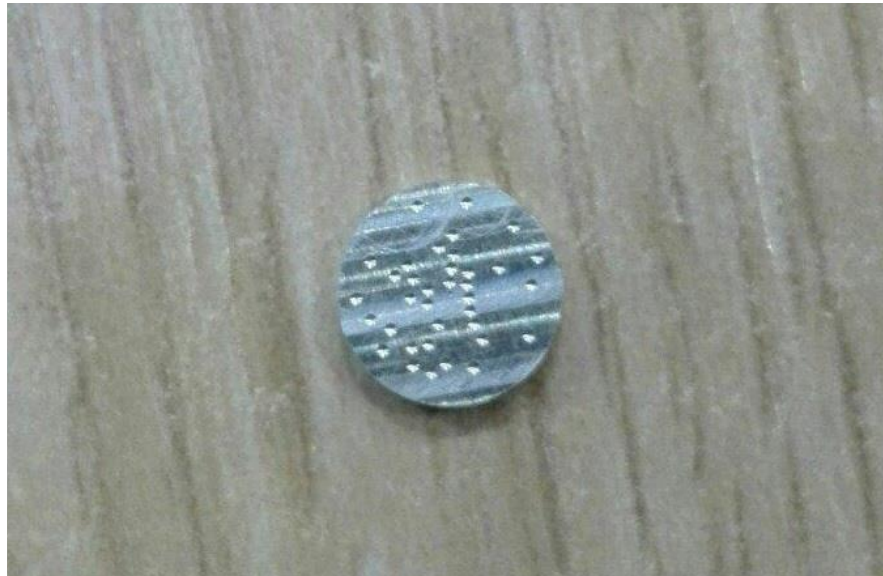
Figure 2.1: Example of a single disk used in the experiment with the artificial pores drilled on the top face
