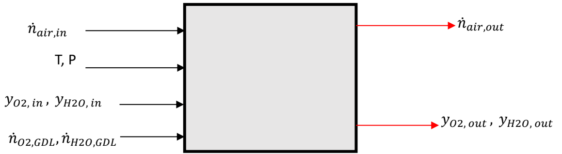
Figure 19 cathode channel model scheme
