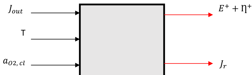
Figure 15 Cathode catalyst layer model scheme
