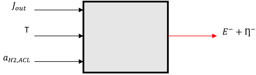
Figure 16 Anode catalyst layer model scheme
