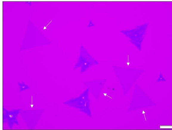
Figure 4.3: Optical image of WS 2 mono- and few-layers. The monolayers are indicated with white arrows. Scale bar: 50 \mu\text{m} .
