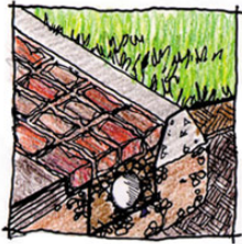
Paving strip with sediment trench
