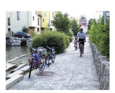
Pervius pavement: In the community, the pavement are paved with pervious asphalt, and the sidewalks also use pervious bricks and recycled granite, successfully reducing the impervious surface from 95% to only 50%.
