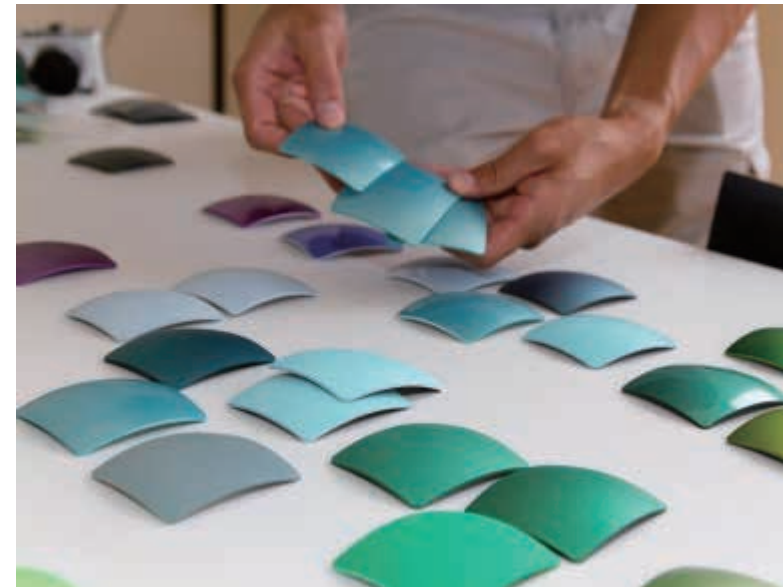
88 Example of Step 6 (Described in Liliana Becerra's book: The fundamental principles of CMF design, Frame Publishers, 2016) A professional is revising colour and finish samples provided by a paint supplier, based on a target sample request.
