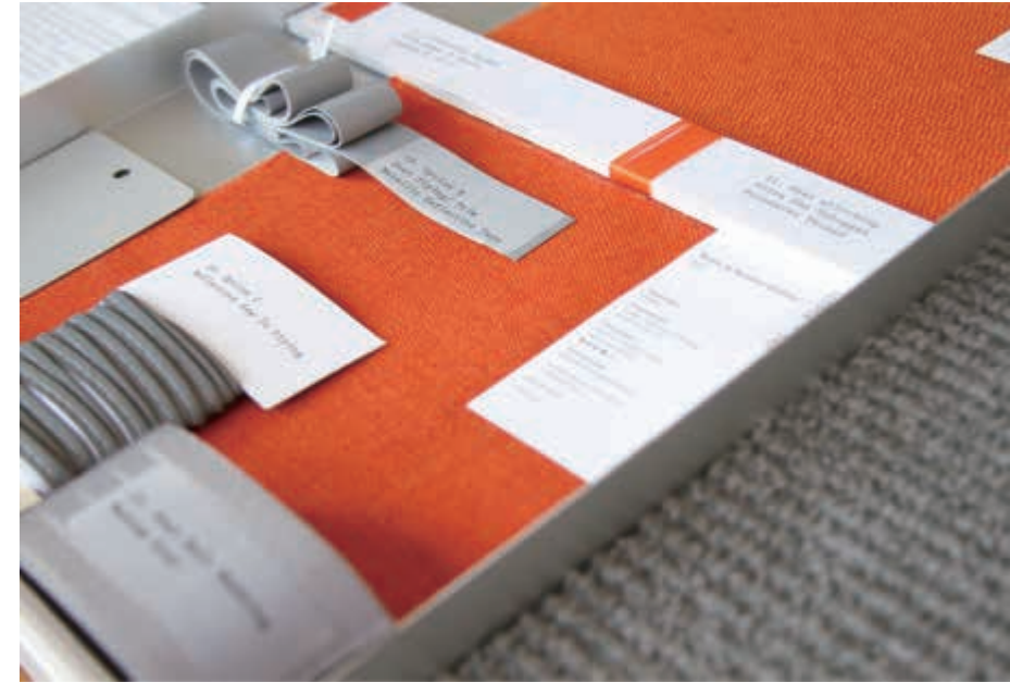
87 Example of Step 5 (Described in Liliana Becerra's book: The fundamental principles of CMF design, Frame Publishers, 2016) Detail of a CMF palette targeting a collection of airplane seat covers, showcasing different materials with their corresponding samples and numbered specifications. Project by Studio Liliana Becerra Inc. for Zodiac Aerospace.
