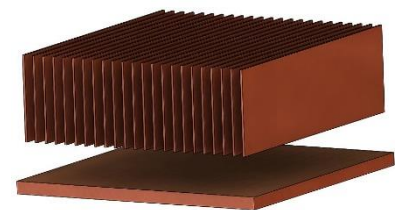
4: Heatsink with separated base
