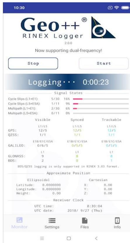
Figure 3.6: Geo++ RINEX Logger interface
