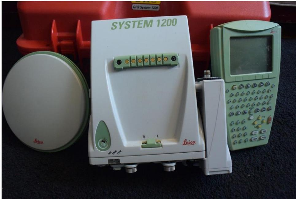
*Figure 3.1: Leica GRX1200 and AX1202 GG antenna*
