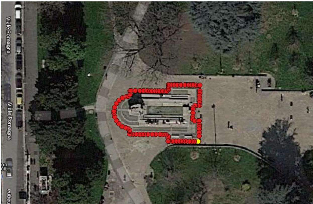
*Figure 4.2: Estimated point locations around the fountain (in red) and estimated starting point location (in yellow)*
