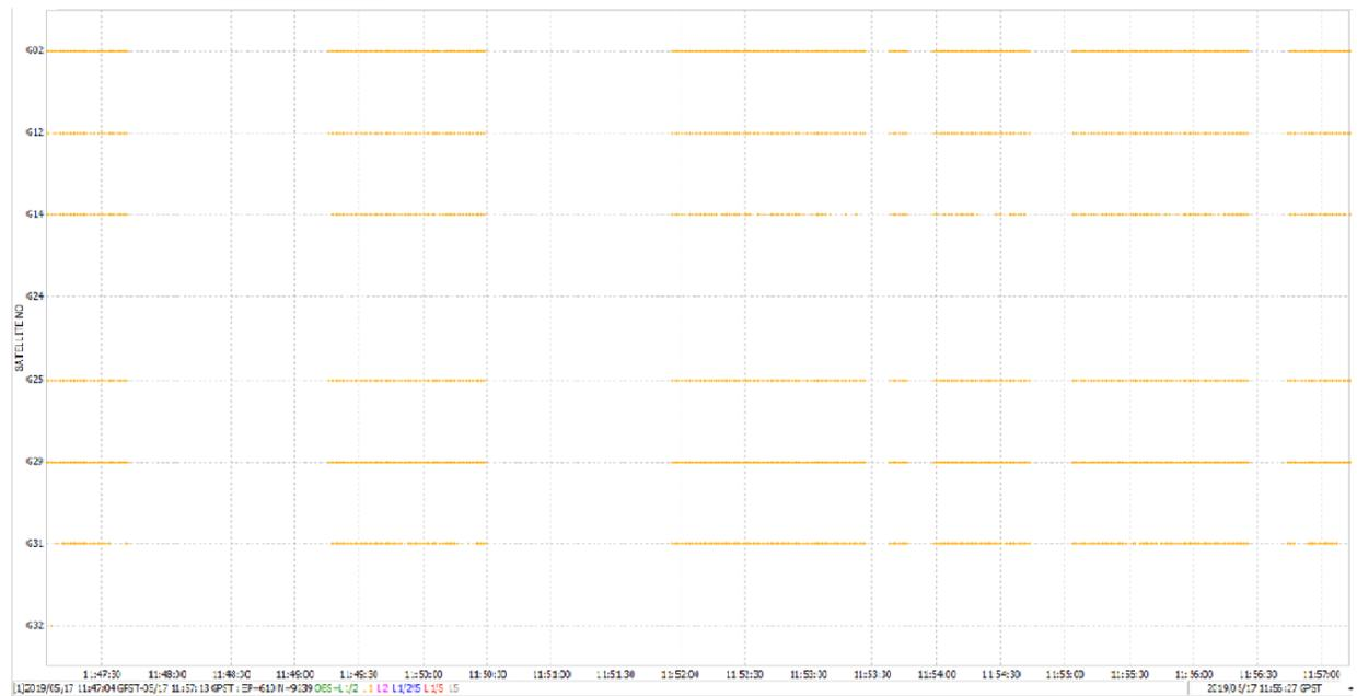
Figure 5.25: Discontinuity problem in the L1 phase observations present in data acquired from Geo++ RINEX Logger for Point 1.
