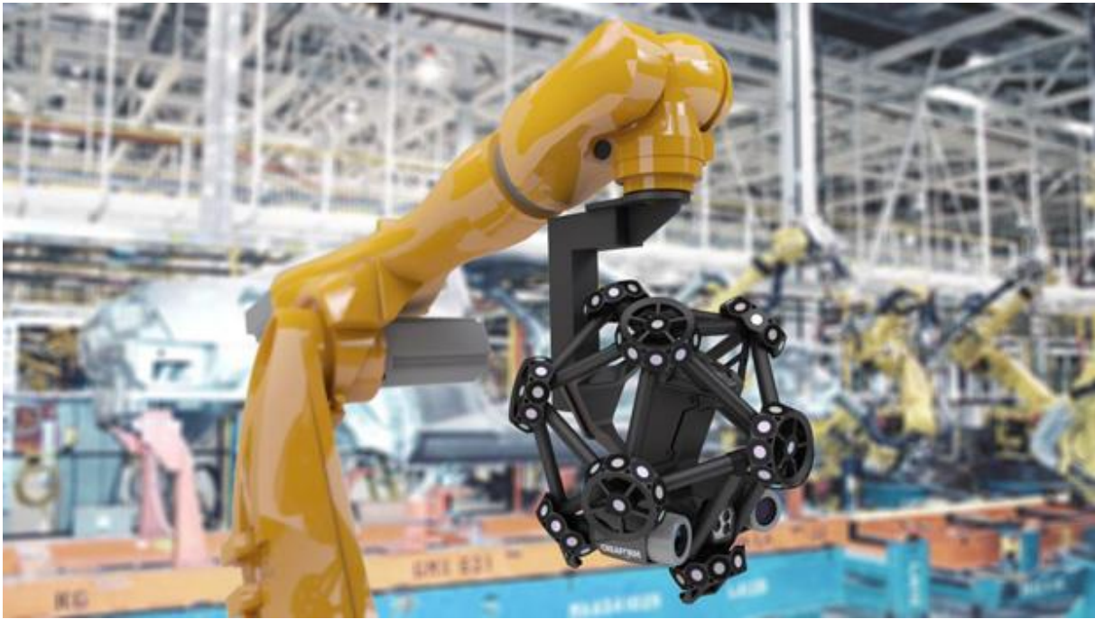
Figure 25. MetraScan 3D laser scanning tool [13]
