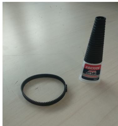
Figure 4.15: A picture of the Belt with the glue used to close it at the proper length
