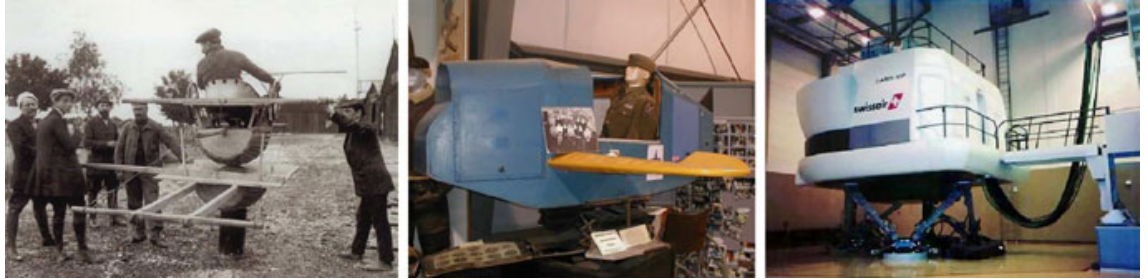
Figure 2.9: History of flight simulation devices: Early synthetic flight training device from 1910, Link Trainer from the 1930s, Contemporary high fidelity flight simulator
