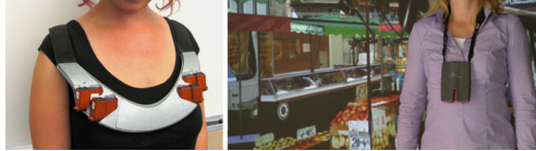
Figure 3.9: Wearable olfactory displays. (a) ICT Scent Collar; (b) Sniffman in combination with virtual marketplace
