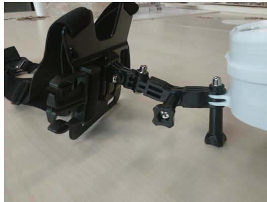
Figure 4.9: The Chest Harness linked to the Jointed Hook screwed with the Case
