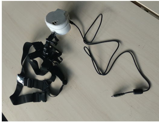
Figure 6.14: The Olfactory Display mounted and ready to be used
