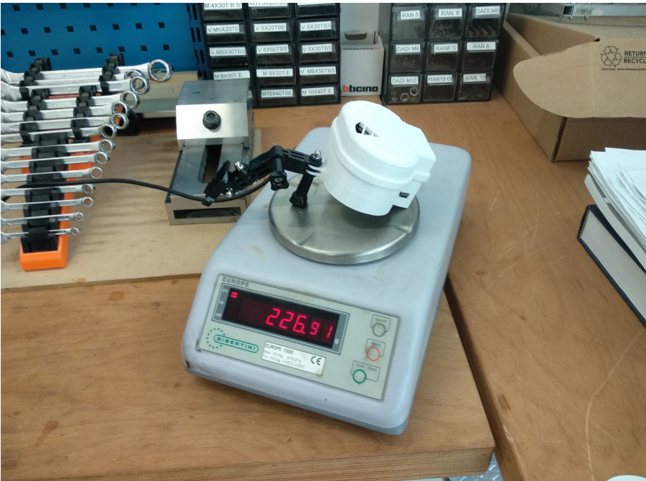
Figure 6.16: The total weight of the prototype measured with a scale
