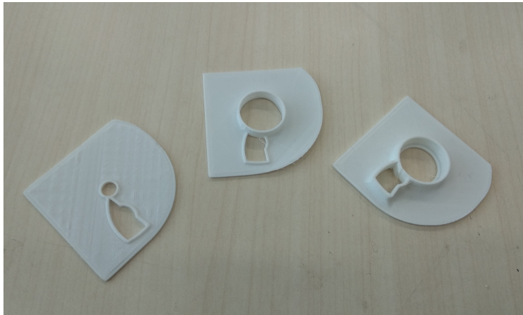
Figure 8.4: The evolution of the Revolver Plate shape from left to right
