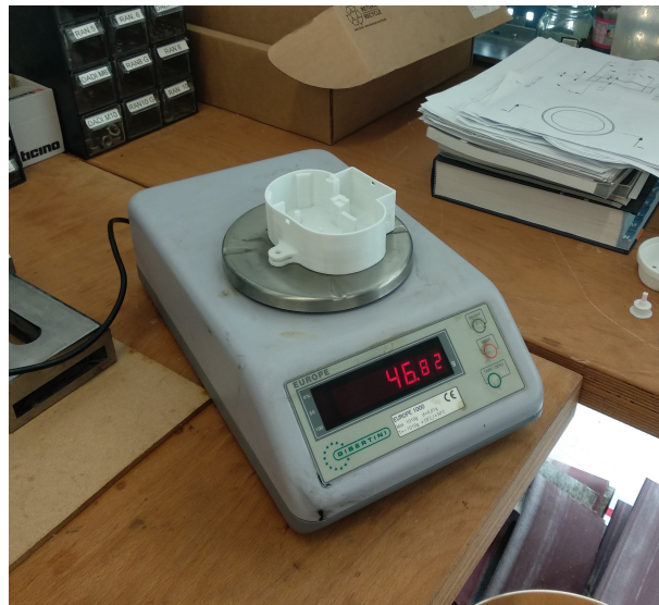
Figure 6.15: The weighing operations to calculate the material consumption
