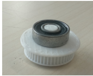
Figure 6.1: The Driving Pulley insertion in the ball bearing
