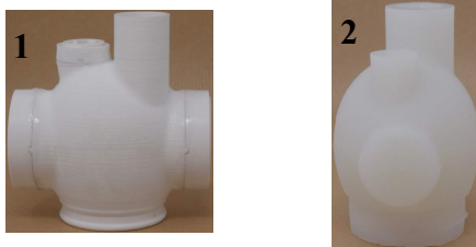
Figure VI: 1) Rigid version in PLA. 2) Flexible version in in PRO-LASTIX 20.
