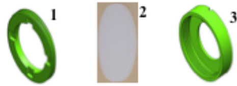
Figure IV: System for the lateral accesses. 1) Screwed element to compress the interposed silicone cylinder with the housing for the screwing tool. 2) Silicone cylinder to be interposed. 3) Screwed element to be fixed to the main body of the rigid atrium and with the support surface for the silicone cylinder.
