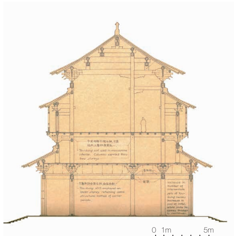
Fig. 4.45 Section of Kui Wen Pavilion (Library Building) Source: Sicheng Liang, A Pictorial History of Chinese Architecture. New Star Press, June, 2017
