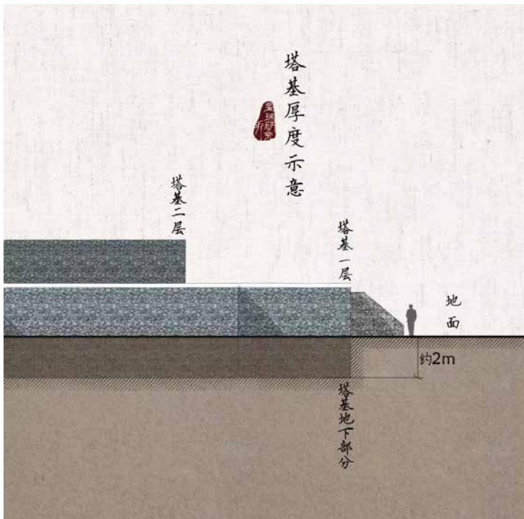
Fig. 4.34 Base of Ying Hsien Wooden Pagoda (below) Source: https:// zhuanlan.zhihu. com
