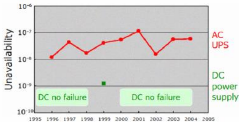
Figure 2.6 - Reliability field data of AC and DC power supply [41]
