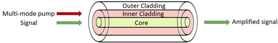
**Figure 2.2.2:** Cladding pumped, double-clad fiber amplifier.
