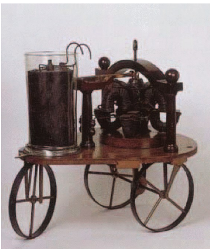
Fig. 3 Stratingh's small electric car
