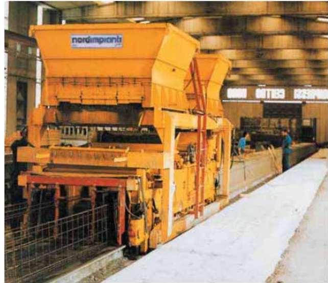
Figure 5.2.2 Vibratory finishing machine for the production of precast reinforced concrete. Source: ASSAP
