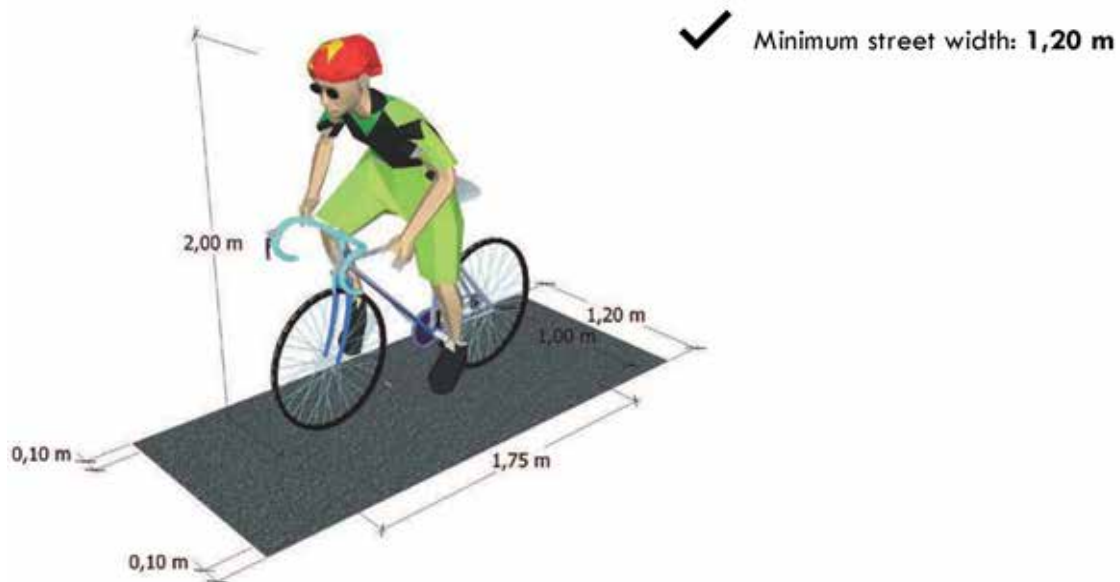
Figure 3.1.4 Minimum dimensions for a cycle path. Source: Morar Carioca, 2010
