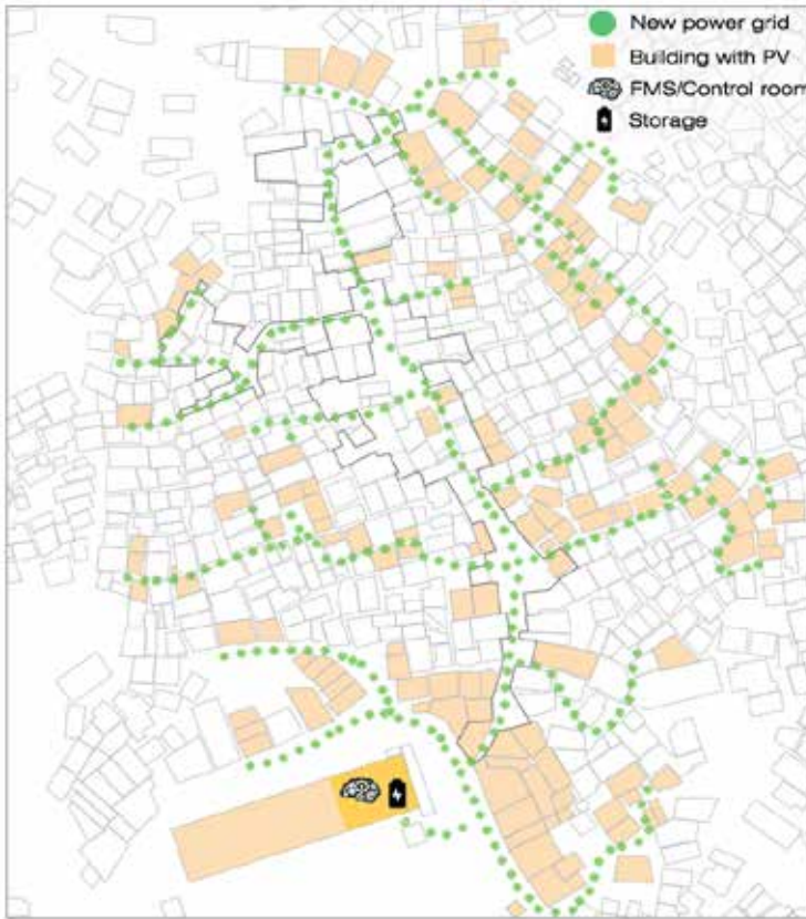
Figure 3.2.14 Area 1 new power grid: buildings with PV panels. Courtesy of PolimiparaRocinha
