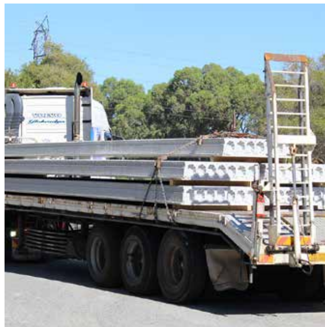
Figure 5.2.3 Transportation of hollow core precast slabs. Source: bgcprecast.com.au
