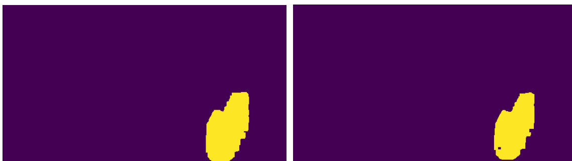
Figure 4.33 On the left, the mask created upon MCV's method is implemented. On the right, the mask acquired after binary filtering operations.
