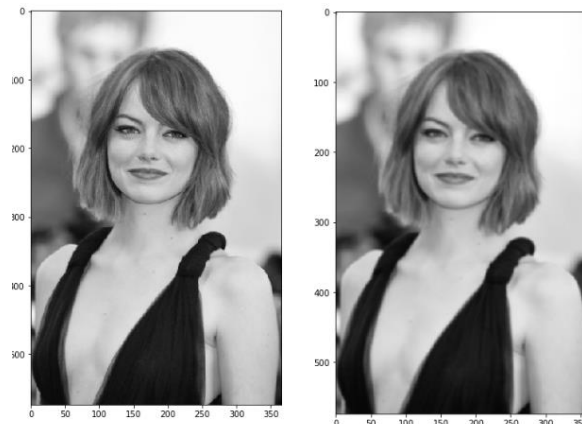
Figure 3.22 Gaussian filter effect on stock image
