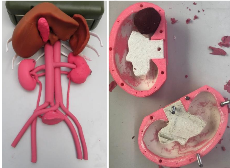
Figure 5.6 On the left, Phantom kidney setup. On the right, kidney molds. Some blood vessel-like details were drawn on the kidney phantom manually with a color marker.
