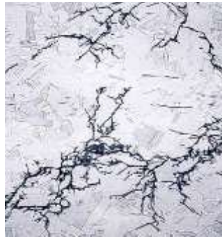
Figure 20.B Start of stress corrosion cracking. (Kamnik, April 2008)
