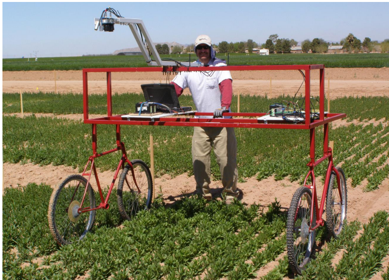
Figure 2.16: View of the proximal sensing cart in a field of camelina. (Image source [24] )
