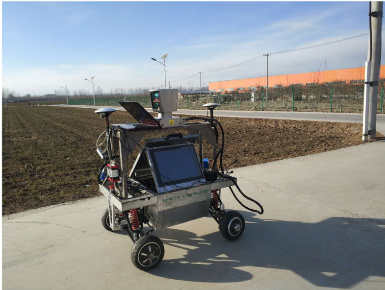
Figure 2.2: Qiu et al. developed UGV with the Velodyne HDL64E-S3 LiDAR sensor. (Image source [11] )
