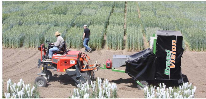
Figure 2.11: BreedVision sensor platform during outdoor measurements in the field. (Image source [19] )
