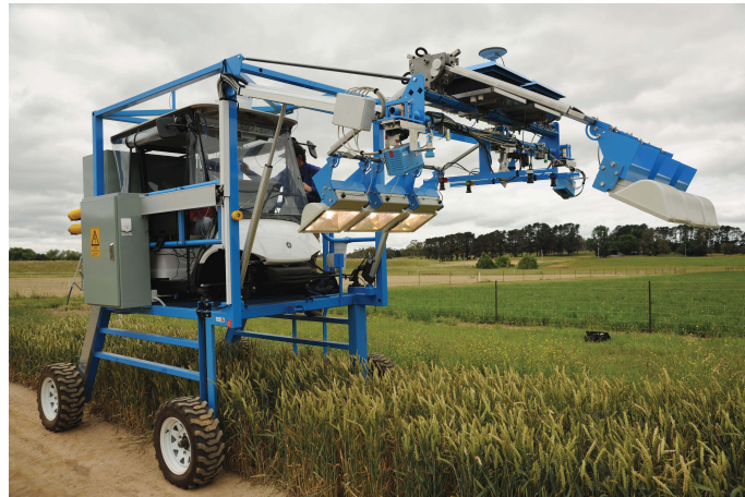
Figure 2.9: The Phenomobile tractor-based system investigated by Deery et al. (Image source [16] )
