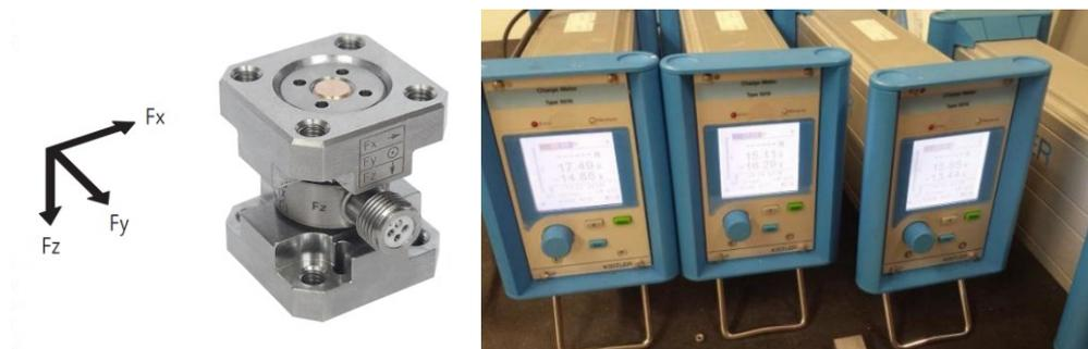
**Figure 47.** Forces acquisition set up: (a) load cell, (b) channel x, y and z.
