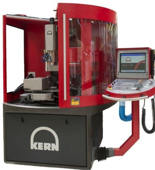
*Figure 45. Kern EVO 5-axis CNC machining centre.*
