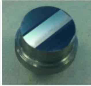
**Figure 33.** Machined mould insert [25].
