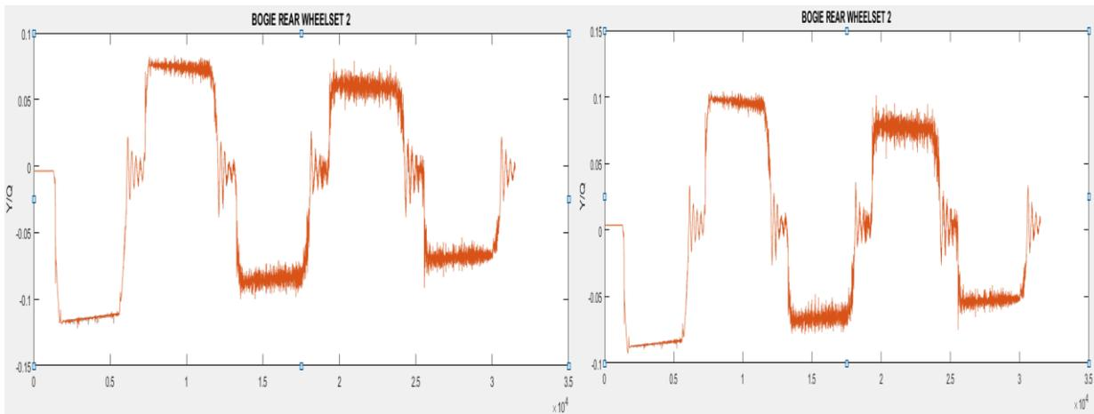
**Fig.50 Quotient of lateral over vertical forces**
