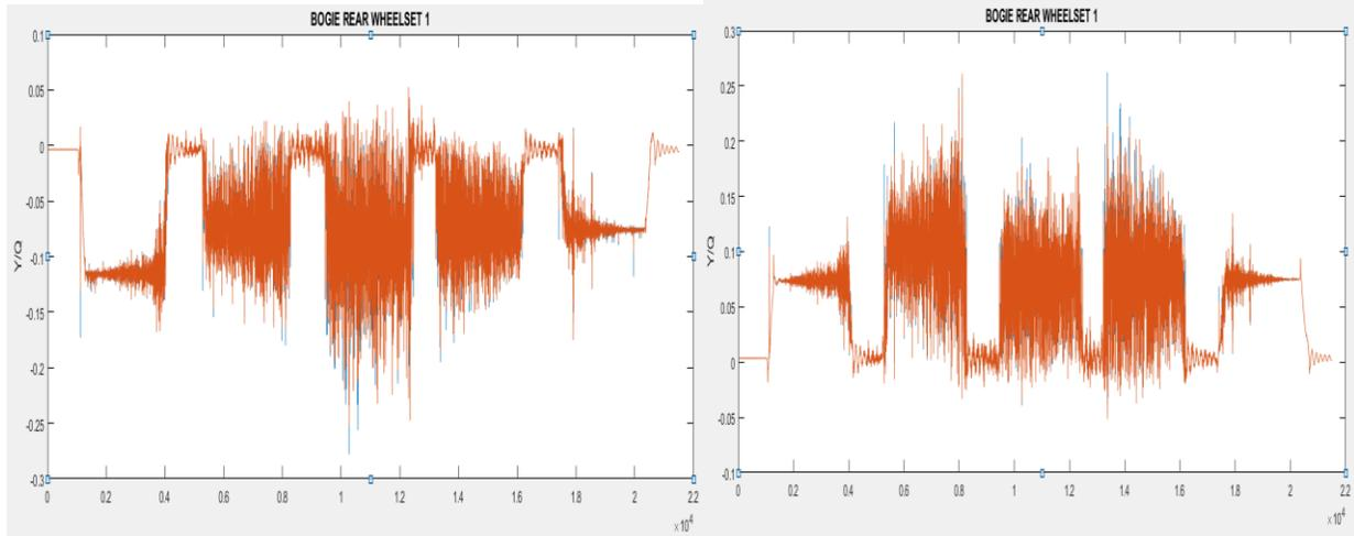
**Fig.28** Quotient of lateral over vertical forces (Y/Q)
