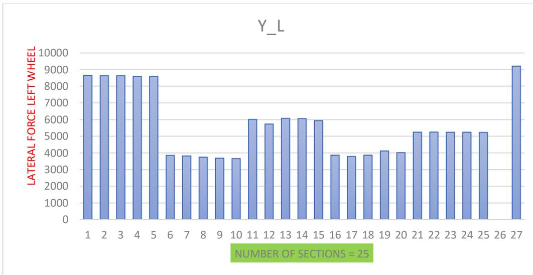
**Fig.5.19 Lateral force Y (Right and left wheel)**
