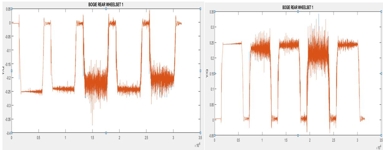
**Fig.46 Quotient of lateral over vertical forces (Y/Q)**
