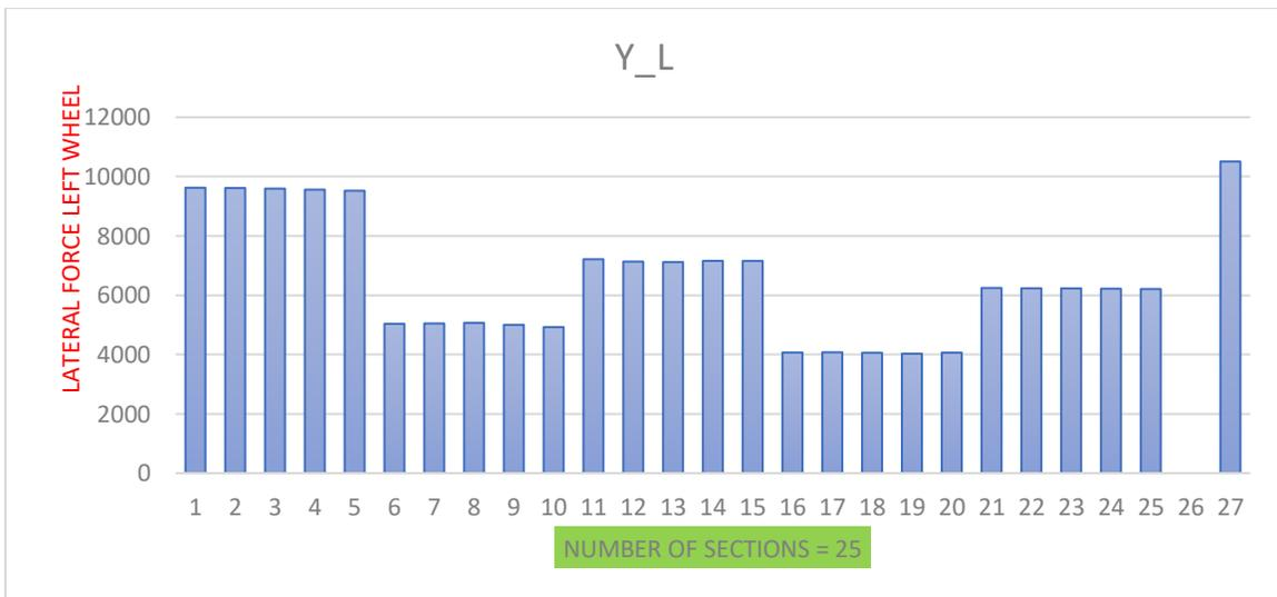
**Fig.5.23 Lateral force Y (Right & Left wheel)**
