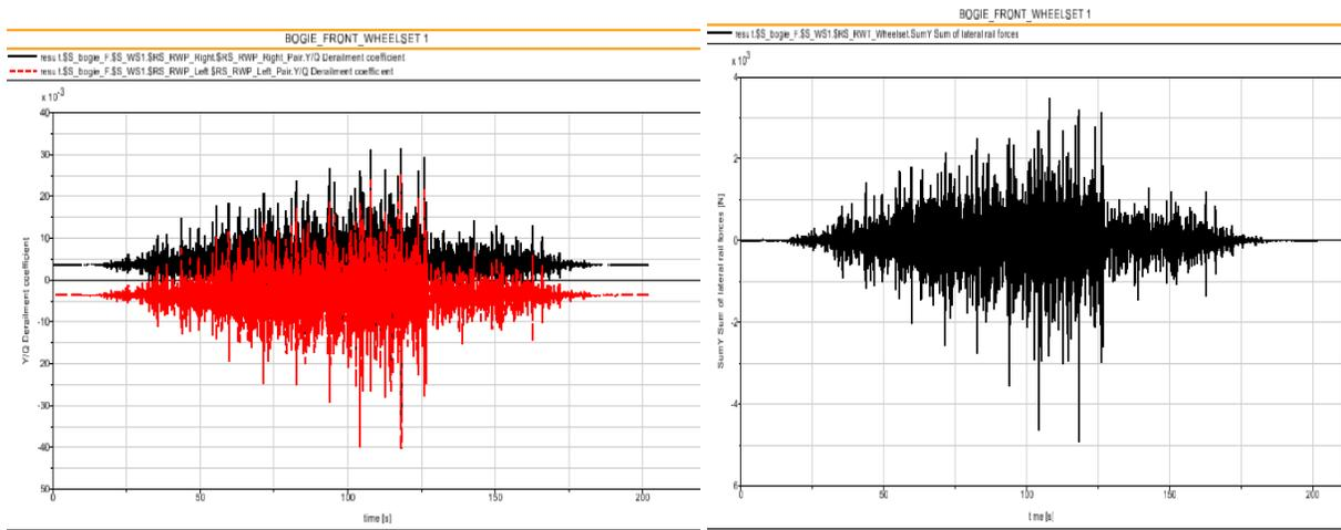
Fig.2 Quotient of lateral and vertical forces (Y/Q) Fig.3 Sum of lateral forces wheelset 1
