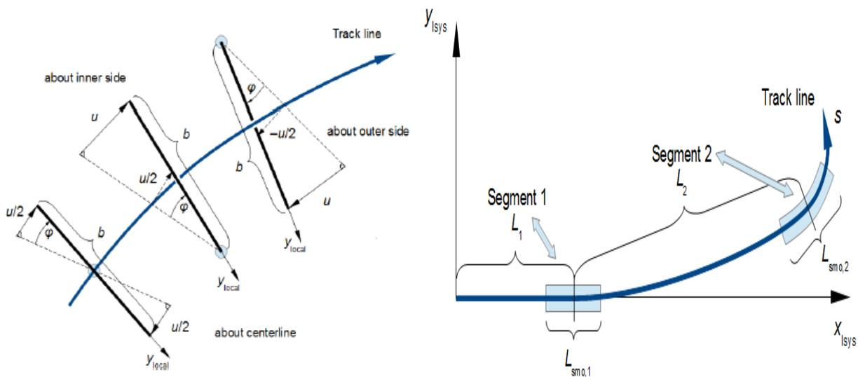
A positive super-elevation corresponds to a right-hand curve and negative super-elevation corresponds to a left-hand curve.
