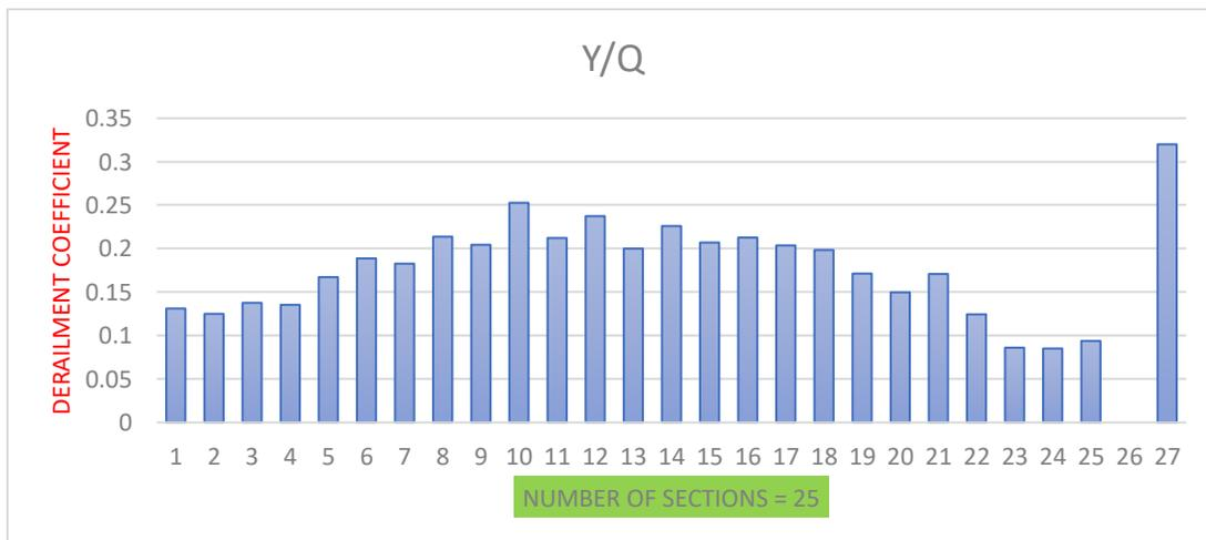
**Fig.5.20 Derailment coefficient (Running safety)**
