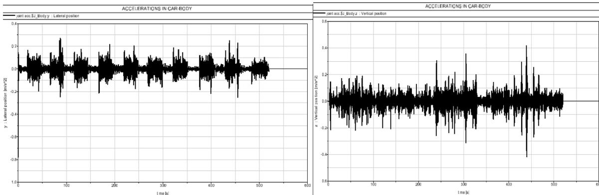
**Fig.4.83 Lateral and vertical acceleration car-body**
