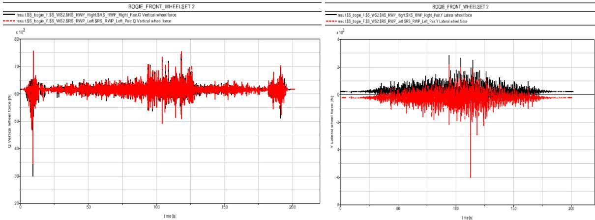
**Fig.4 Vertical force Q & Lateral force Y wheelset 2**
