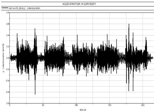
**Fig.33 Lateral acceleration car-body**
