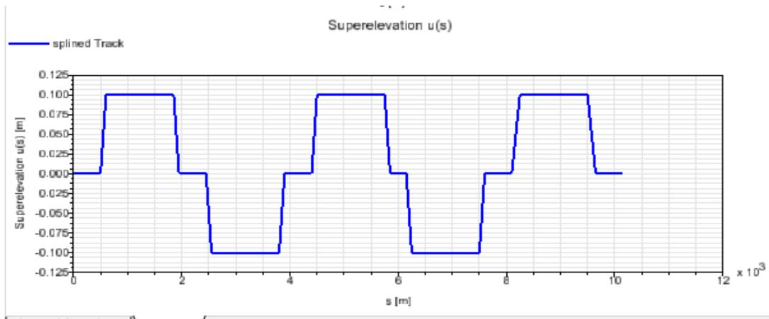
**Fig.3.25 Super-elevation layout model test zone 2**
