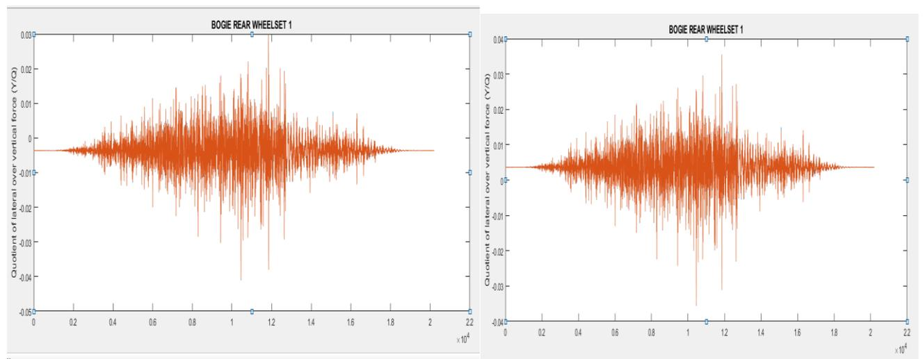
**Fig.11 Quotient of lateral over vertical force (Y/Q)**
