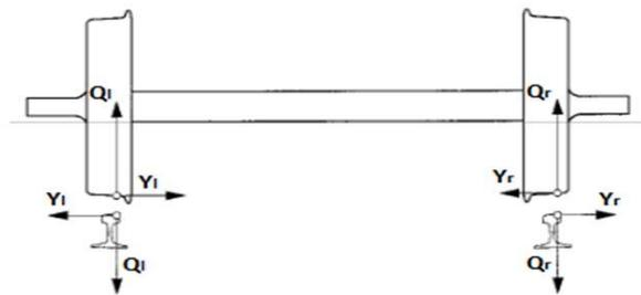
**Fig.2.1 Wheel-rail contact**
