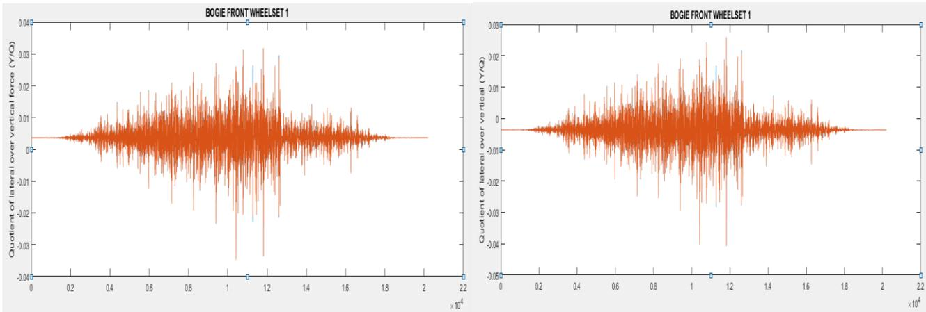
Fig.3 Quotient of lateral over vertical force (Y/Q)
