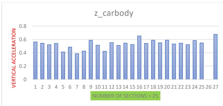
**Fig.5.26 Vertical acceleration (Ride characteristics)**
