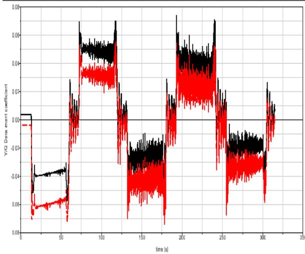
**Fig.41** Quotient of lateral over vertical force (Y/Q)
