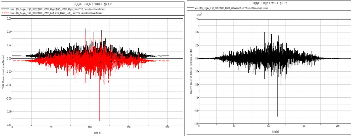
**Fig.5 Quotient of lateral and vertical forces (Y/Q) Fig.6 Sum of lateral forces wheelset 2**
