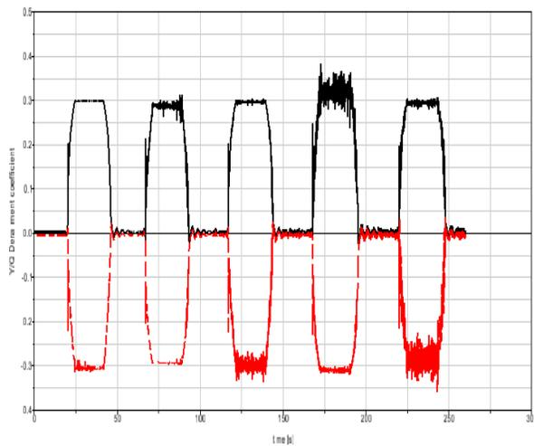
**Fig.62** Quotient of lateral over vertical force (Y/Q) wheelset 1
