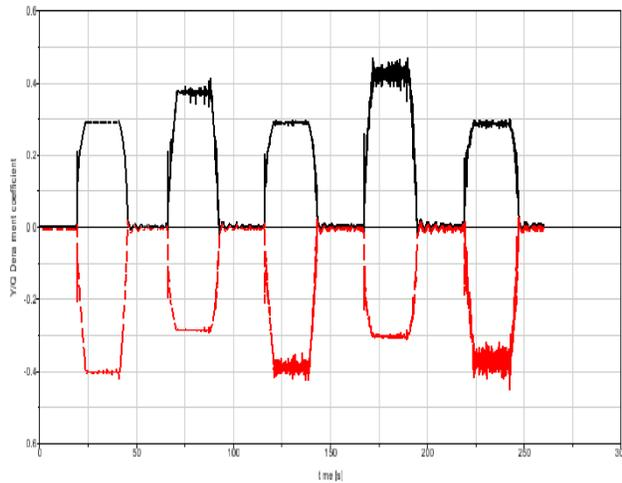
Fig.54 Quotient of lateral over vertical force (Y/Q)
