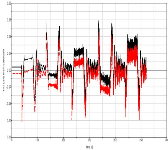
**Fig.58** Quotient of lateral over vertical force (Y/Q)
