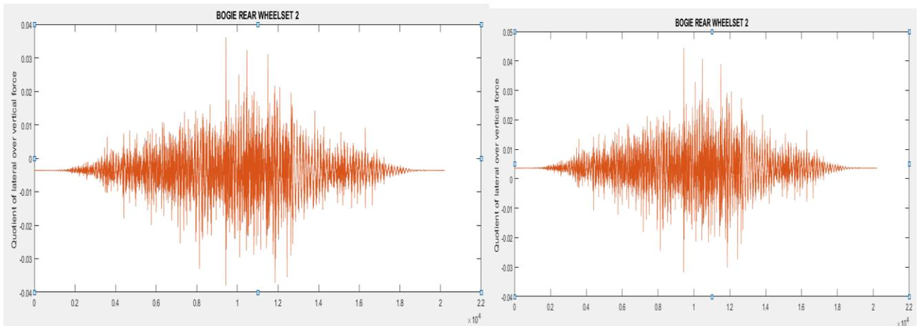
Fig.15 Quotient of lateral over vertical force (Y/Q)
