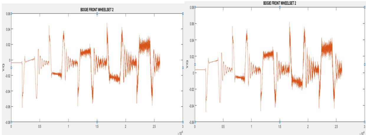
Fig.60 Quotient of lateral over vertical (Y/Q)
