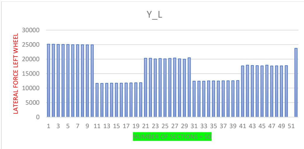
**Fig.5.28 Lateral force Y (Right & Left wheel)**
