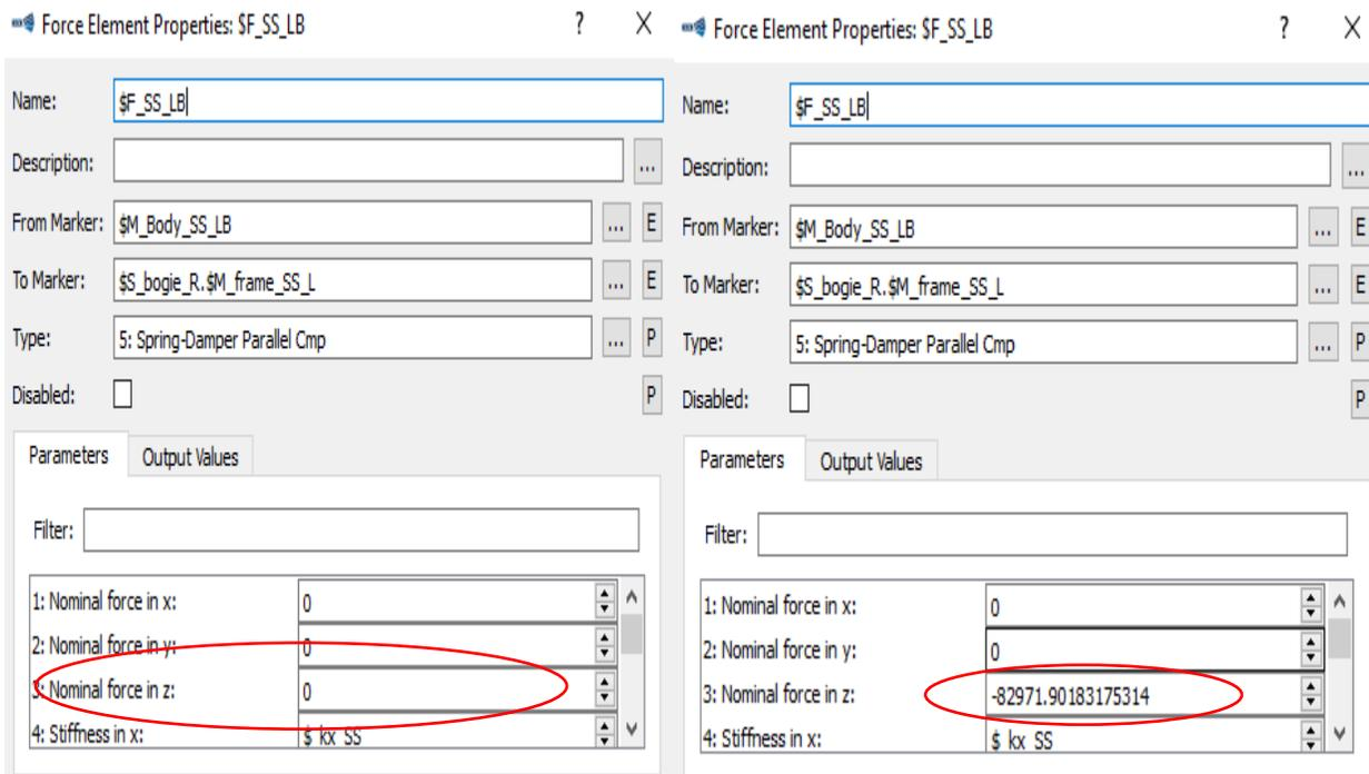
**Fig.3.17 Force elements (Secondary Suspension) Left Back Bogie before and after preload check**
