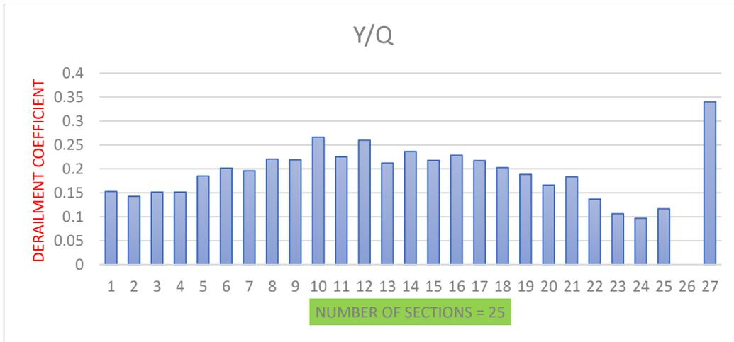
**Fig.5.13 Derailment coefficient (Running safety)**
