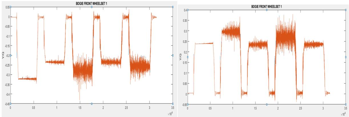
**Fig.38 Quotient of lateral over vertical forces**
