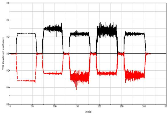
Fig.37 Quotient of lateral over vertical force (Y/Q)
