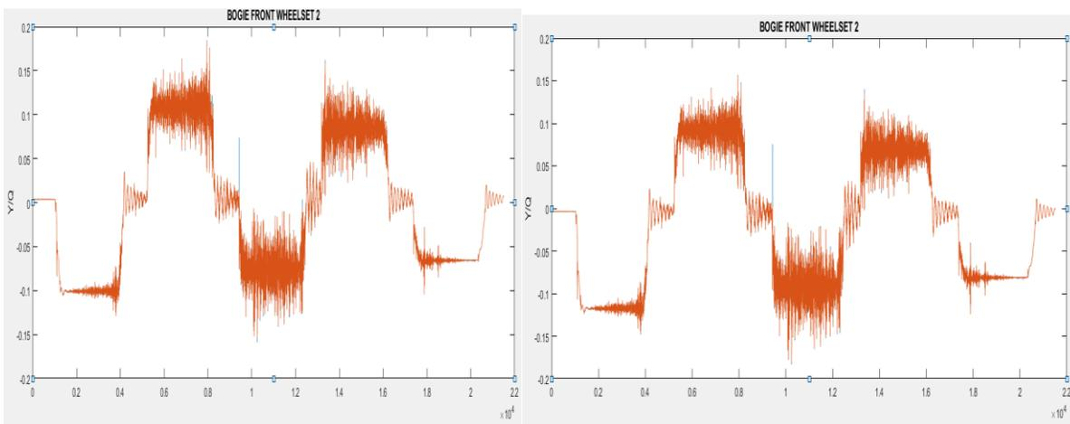
Fig.24 Quotient of lateral over vertical forces
