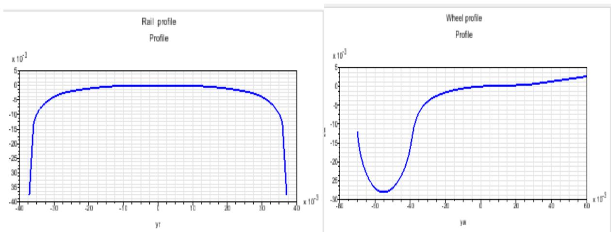
**Fig.3.4 Wheel and Rail profile**
