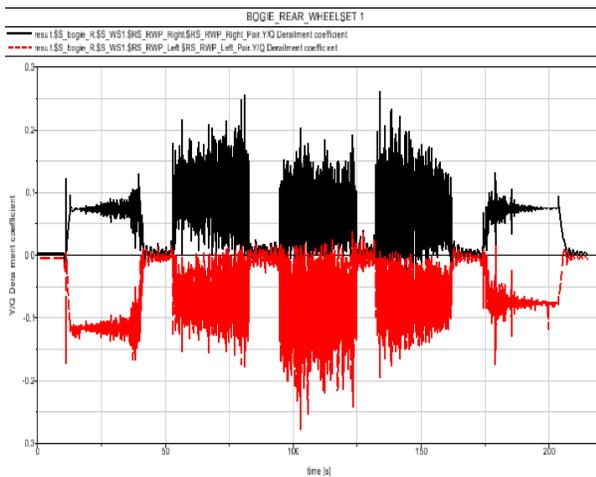
**Fig.27 Quotient of lateral over vertical force (Y/Q)**
