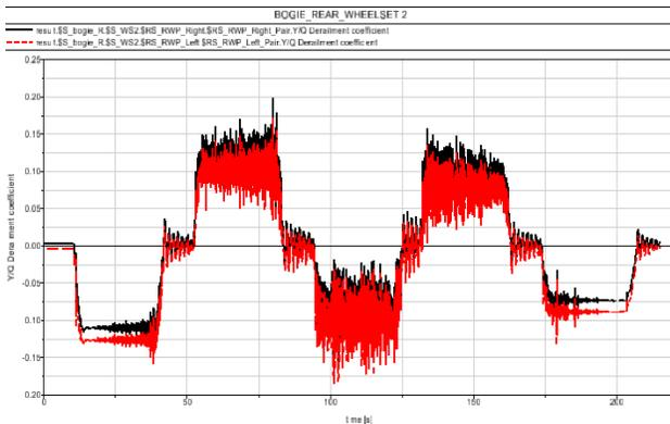
**Fig.31 Quotient of lateral over vertical force (Y/Q)**
