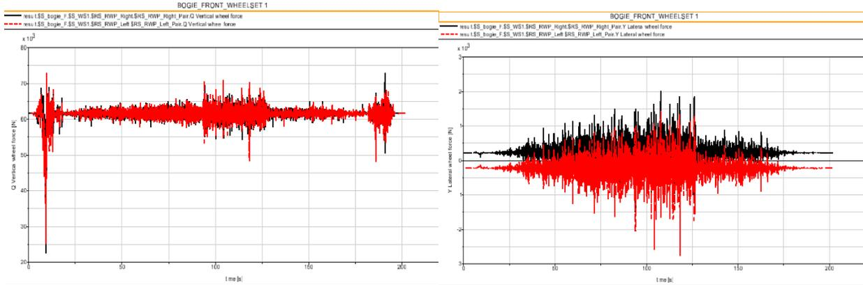
Fig.1 Vertical force Q & Lateral force Y(left and right wheel)
