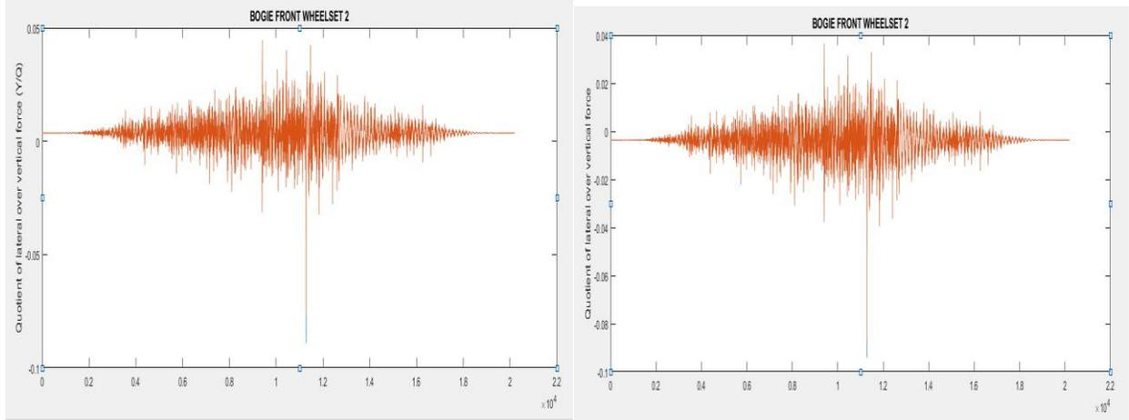
**Fig.7 Quotient of lateral over vertical force (Y/Q)**
