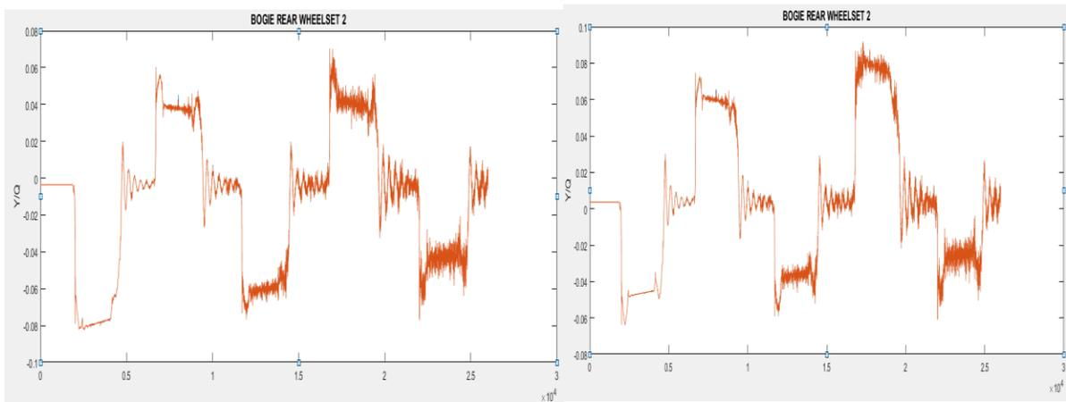
**Fig.68 Quotient of lateral over vertical force (Y/Q)**
