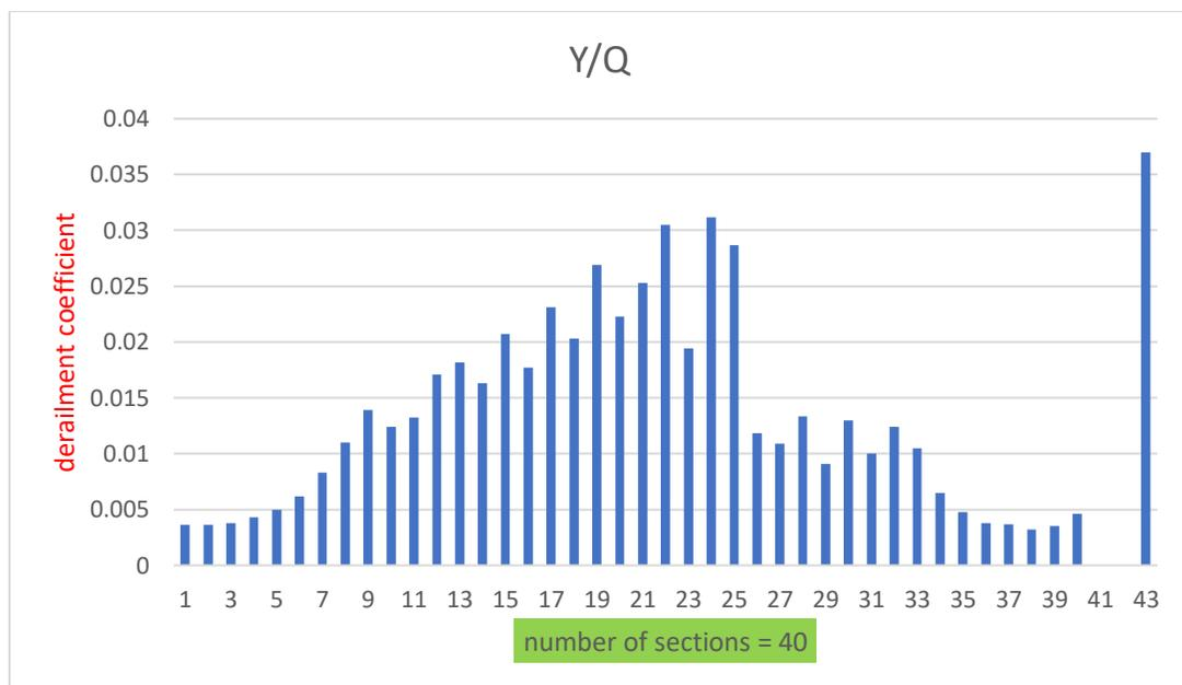
Fig.5.2 Derailment coefficient (Running safety)
