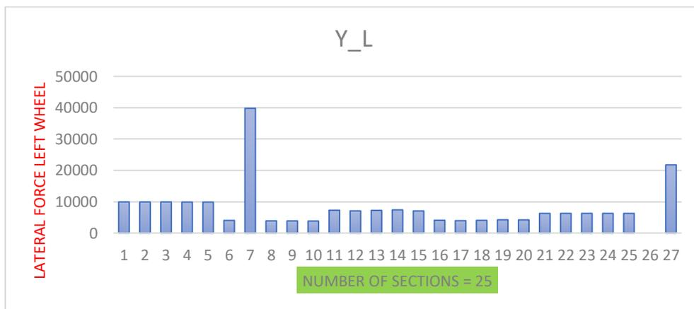
Fig.5.12 Lateral force Y (Right & Left wheel)
