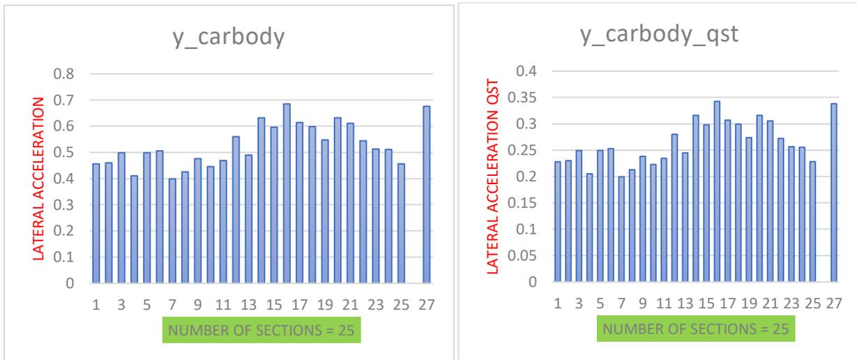
**Fig.5.25 Lateral acceleration (Ride characteristics)**
