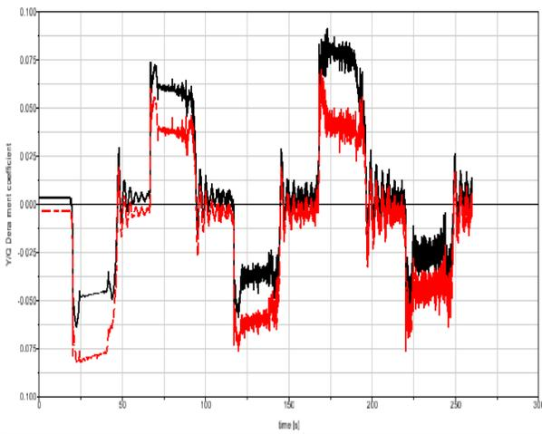
**Fig.66 Quotient of lateral over vertical force (Y/Q)**
