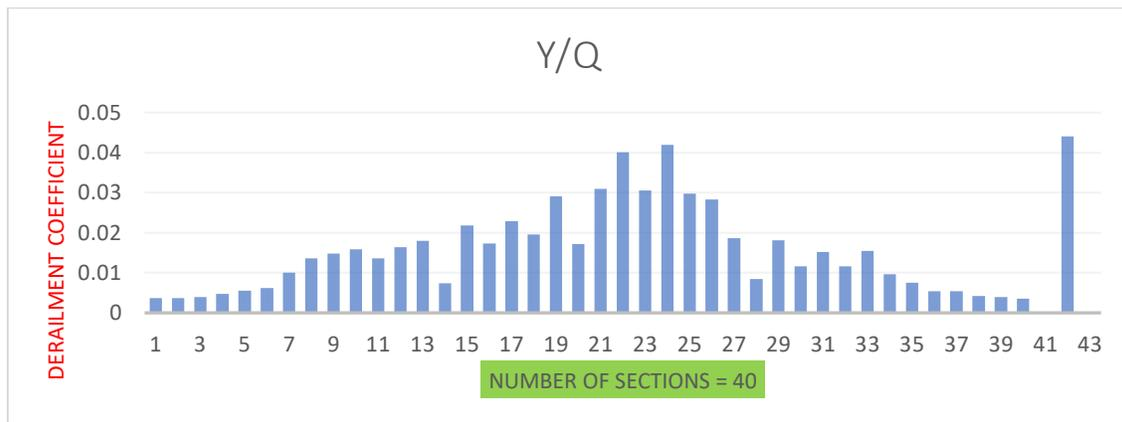
**Fig.5.4 Derailment coefficient (Running safety)**
