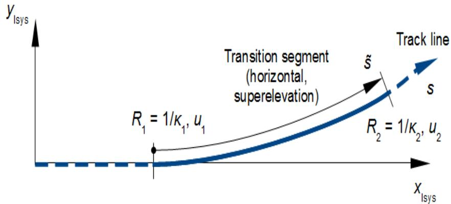
**Fig.3.19 Horizontal track model with transition segment**
