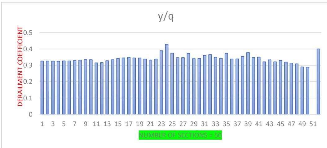
**Fig.5.29 Derailment coefficient (Running safety)**
