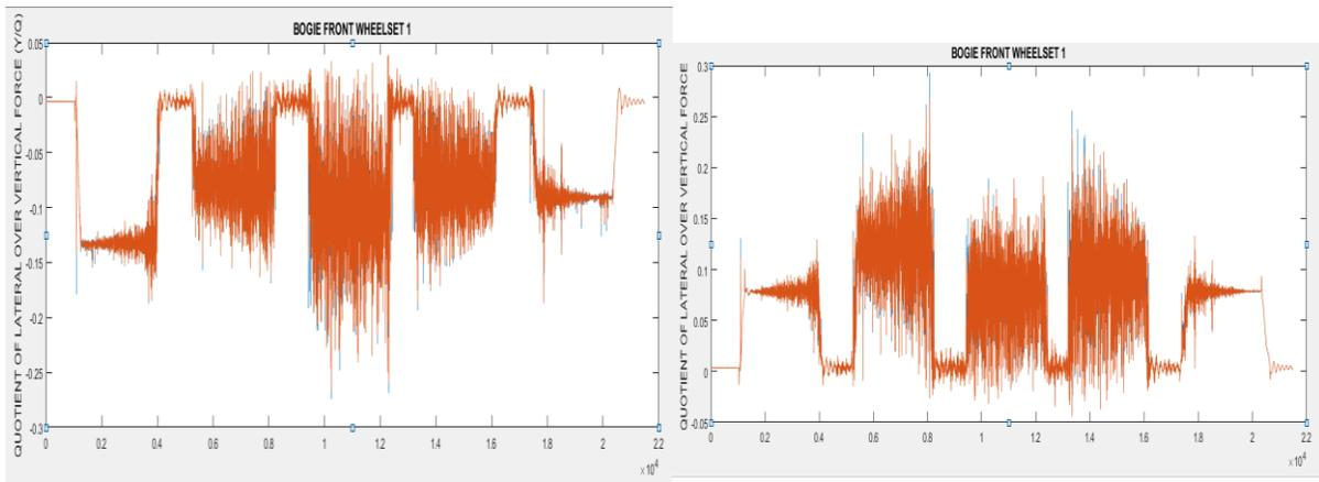
**Fig.20 Quotient of lateral over vertical force (Y/Q)**
