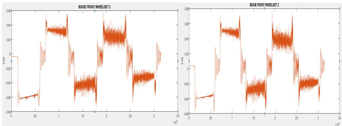
Fig.42 Quotient of lateral over vertical forces
