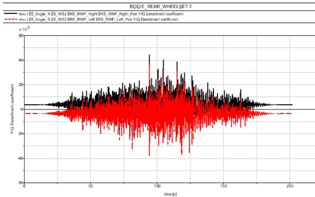
**Fig.13 Quotient of lateral over vertical force**
