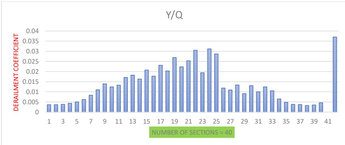
**Fig.5.6 Derailment coefficient (Running safety)**
