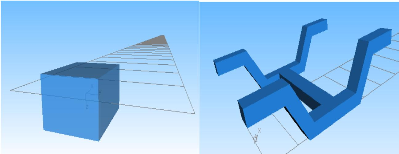
**Fig.3.7 Bogie frame profile**
