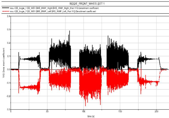
Fig.19 Quotient of lateral over vertical force (Y/Q)
