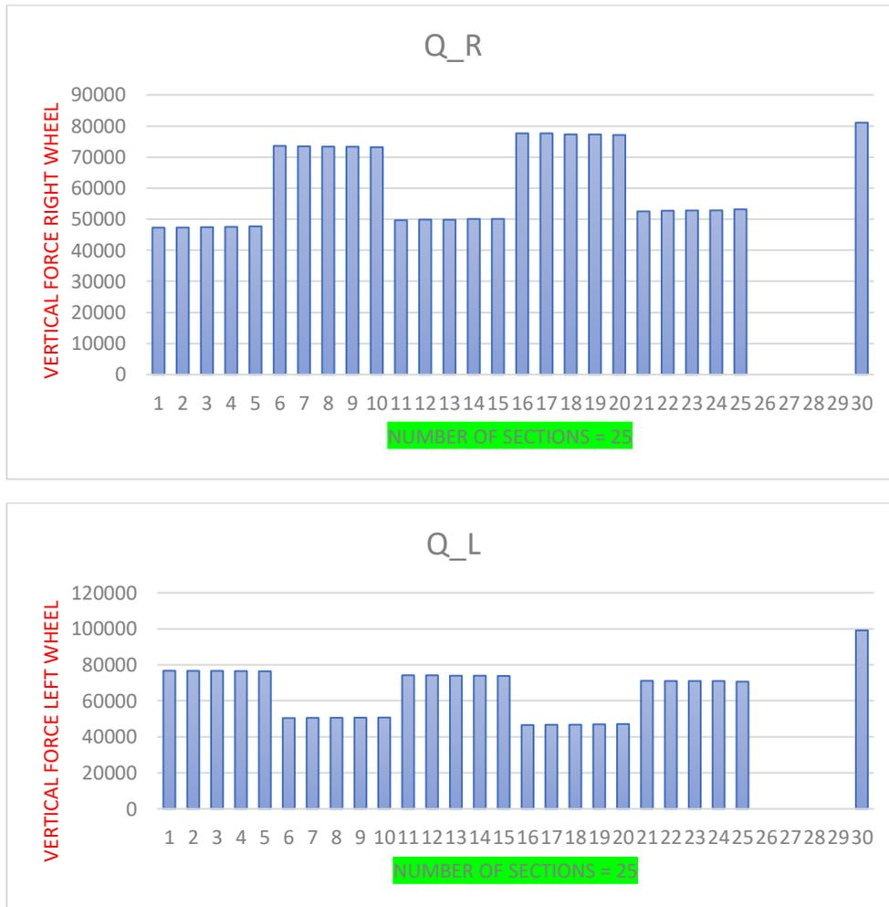
**Fig.5.43 Vertical force Q (Right & Left wheel)**
