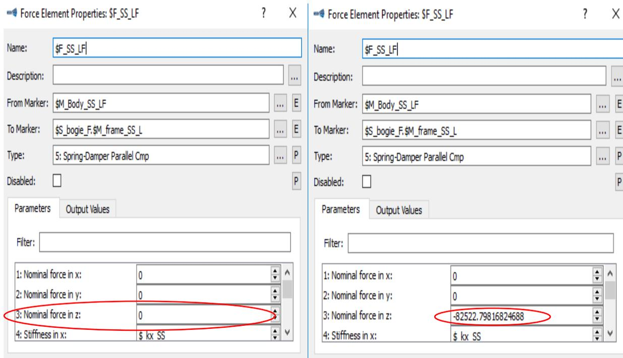
**Fig.3.18 Force elements (Secondary Suspension) Left Front Bogie before and after preload check**
