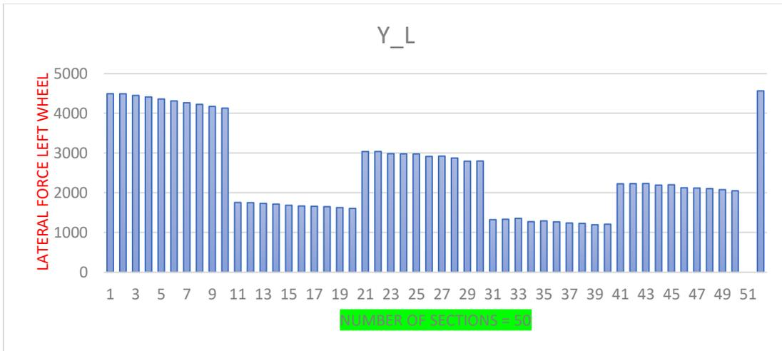
**Fig.5.32 Lateral force Y (Right & Left wheel)**
