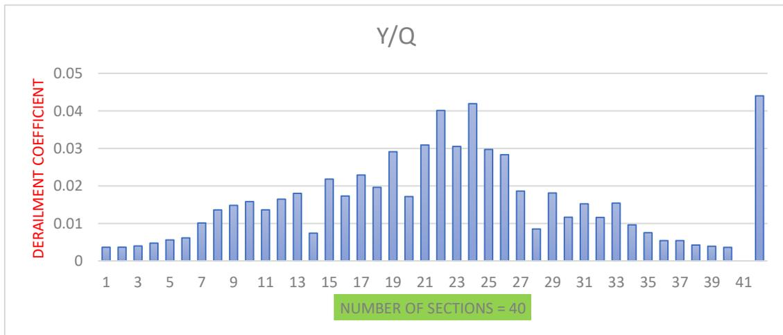
**Fig.5.8 Derailment coefficient (Running safety)**
