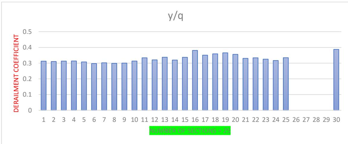
**Fig.5.52 Derailment coefficient (Running safety)**
