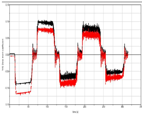
**Fig.49 Quotient of lateral over vertical force (Y/Q)**
