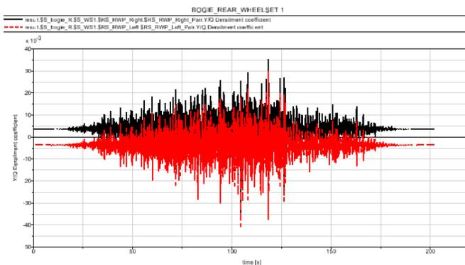
**Fig.9 Quotient of lateral over vertical force (Y/Q) Fig.10 Sum of lateral force wheelset 1**
