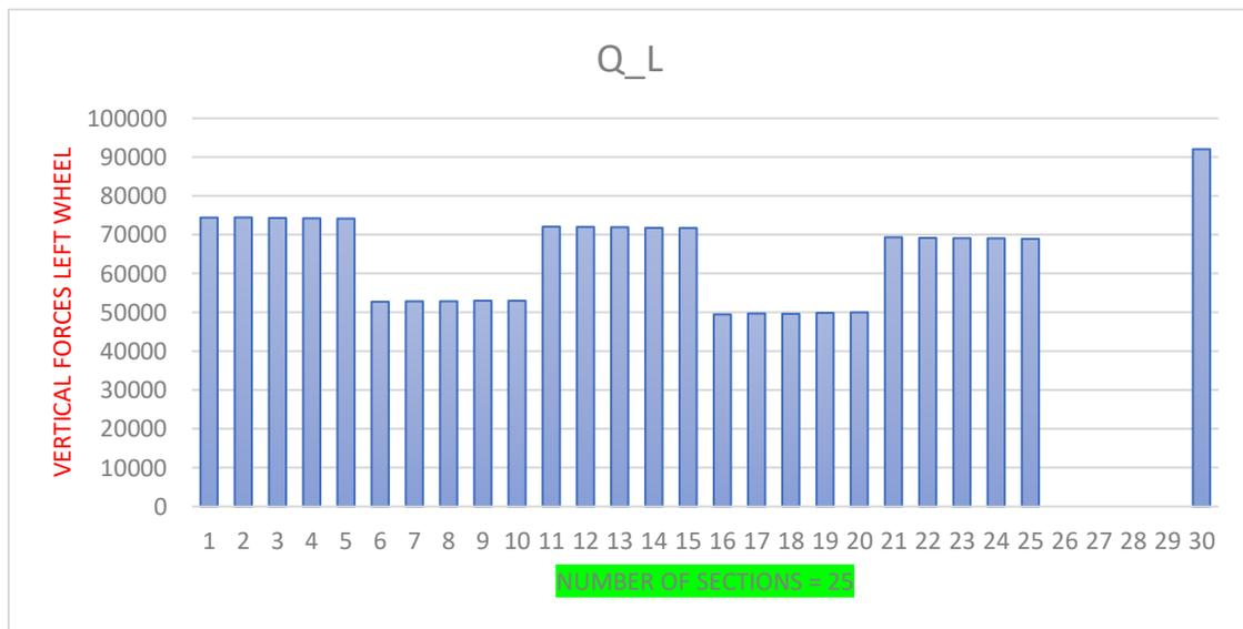
**Fig.5.50 Vertical forces Q (Right & left wheel)**
