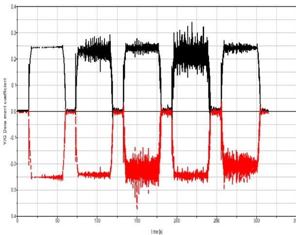
**Fig.45** Quotient of lateral over vertical force (Y/Q)
