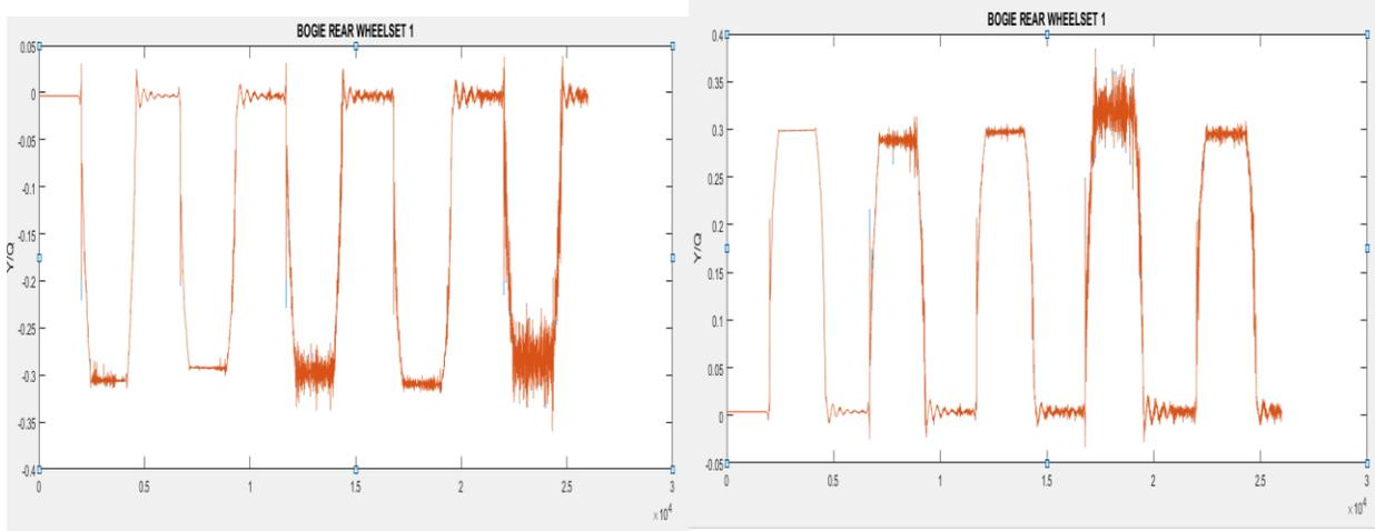
**Fig.64 Quotient of lateral over vertical force (Y/Q)**
