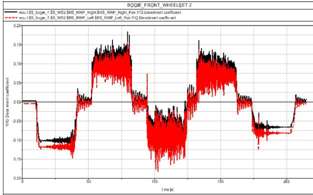
**Fig.23 Quotient of lateral over vertical (Y/Q)**
