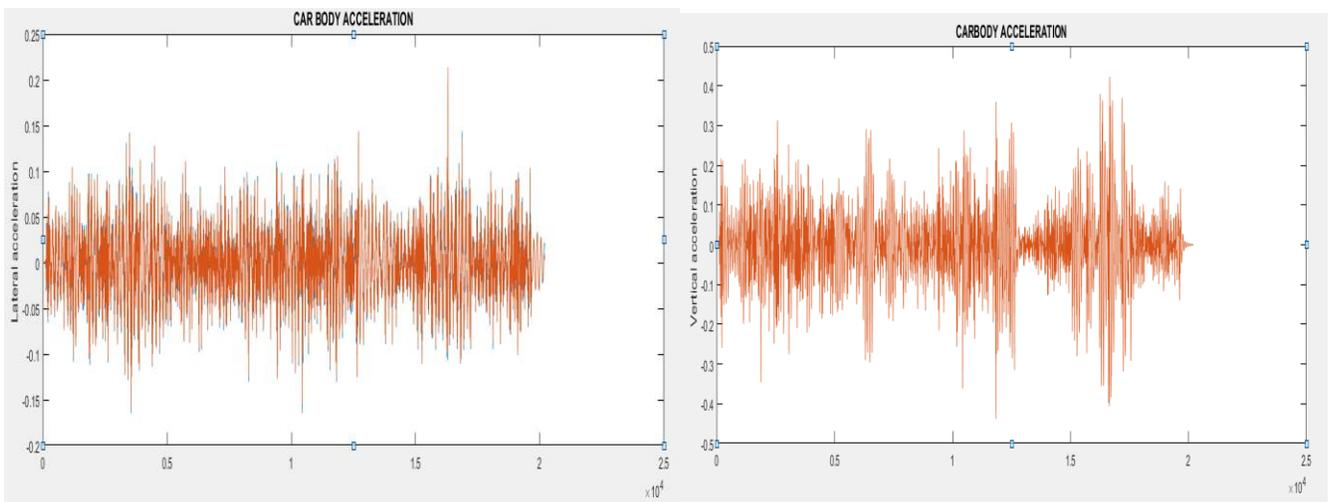
**Fig.17 Car-body acceleration**
