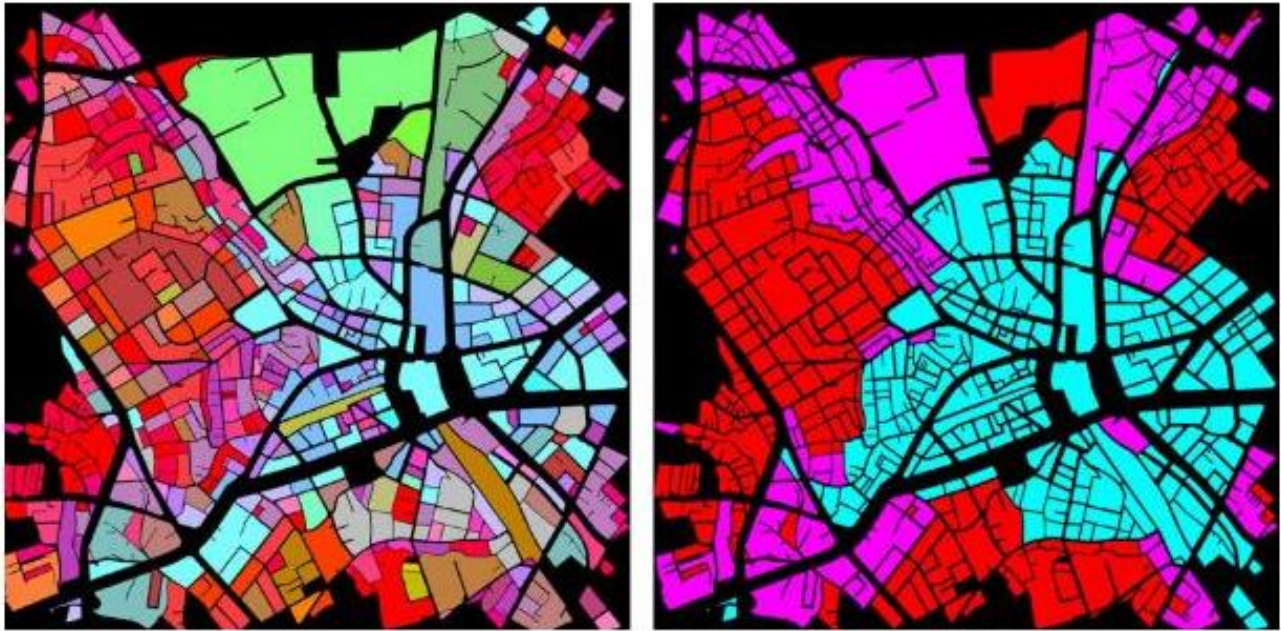
Figure 27 False colour composite made from three morphological variables (left) and governmental specification of land use (right). RGB channels: R = S/V; G = mean building volume; B = volume density Land use: Red = residential blocks; Cyan = commercial blocks; Magenta = mix used blocks (Yoshida & Omae, 2005)
