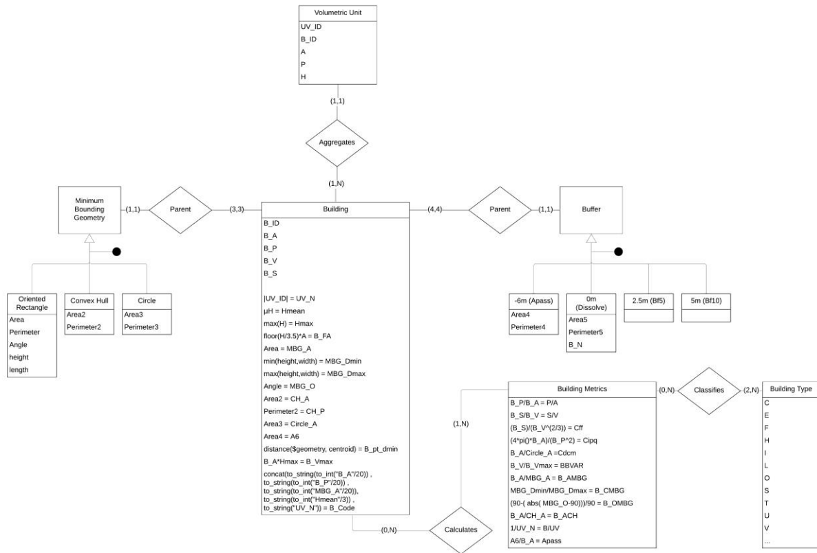
Figure 45 Layer to Metrics. The scheme shows the how to generate attributes and metrics performing spatial operations on Volumetric Unit (Volume input layer). Building attribute set is implemented with the use of ancillary layers and used to generate metrics that allow a classification process.
