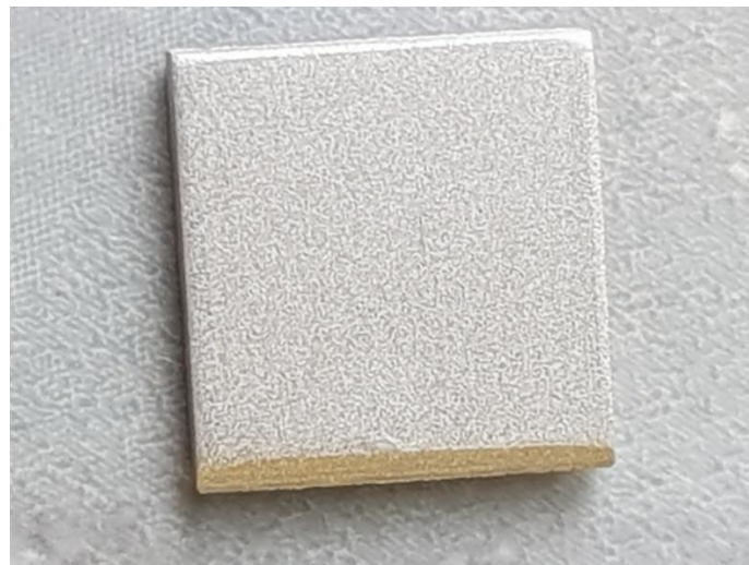
Figure 3.3.11 - Sample of Ti grade 2 after 24 h in 10% v/v oxalic acid at 60°C.
