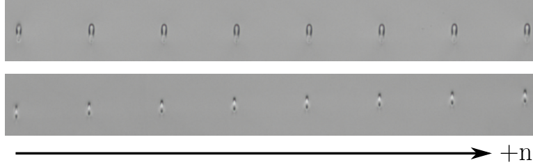
Figure 6.5: Microscope images of the waveguides fabricated for the refractive index optimization. The above waveguides are at 250\ \mu\text{m} from the top surface; below they are at 1\ \text{mm} .
