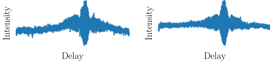
Figure 6.18: Polychromatic fringe pattern as a function of the delay, measured for two different baselines. The output has been recorded from waveguide number 14 of the upper DBC.
