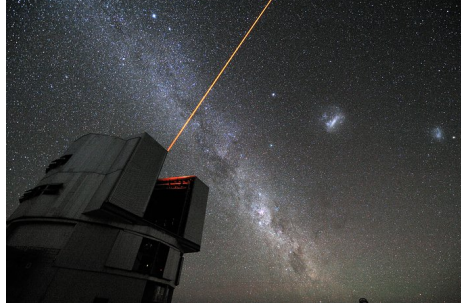
Figure 2.11: Laser-guide star at the Very Large Telescope in Chile. Image from https://www.eso.org/public/ .
