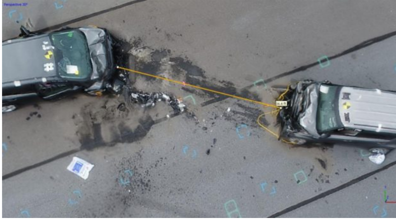
Figure 2.14: Photogrammetry reconstruction of an accident scene.
