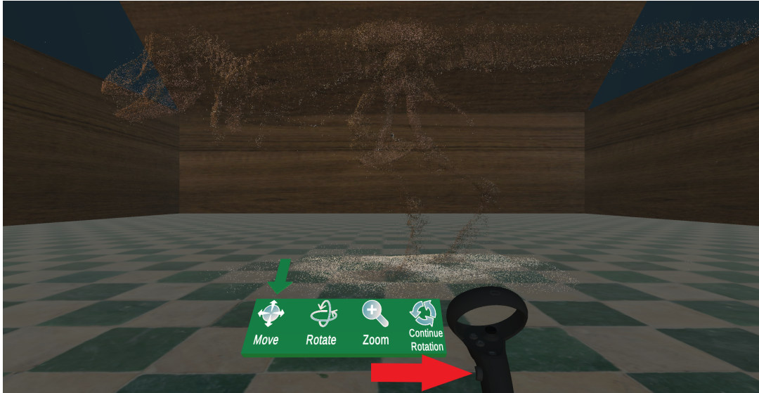
Figure 6.22: Interaction menu open, with a red arrow indicating the controller menu button.
