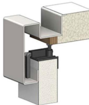
Connection of wall panel to top of box
