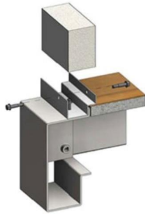
Connection of wall panel to bottom of box
