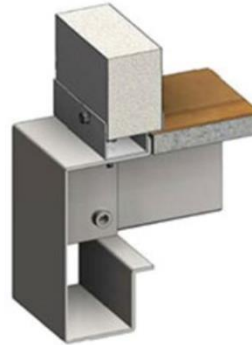
Connection of wall panel to bottom of box
