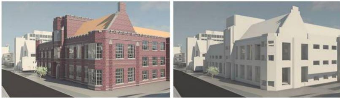
Figure 4.15. BIM models at AIA LOD 500 (left) and AIA LOD 100 (right) [71]
