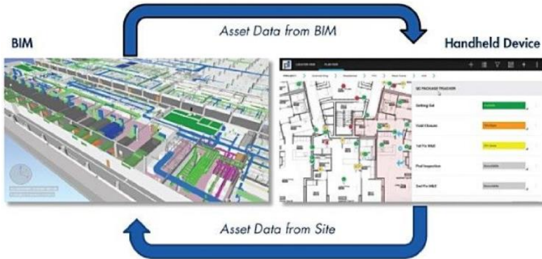
Figure 2.14. Space data in the BIM model of Medina airport displayed on hand-held device (Source: TAV Construction)
