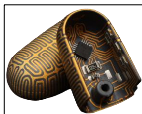
Figure 13: Tactile load cells: artificial fingers
