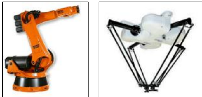
Figure 6: Industrial manipulators: a) Serial robot; b) Parallel robot
